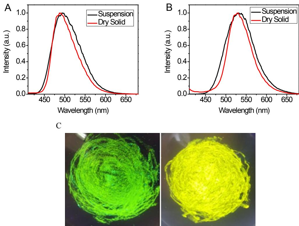
**Fig. S29.** The normalized fluorescence spectra of **6** (A) and **8** (B) in 90:10 H<sub>2</sub>O/THF (V/V) suspension and in dry solid, respectively. (C) Photos of powders of **6** (left) and **8** (right) under a 365 nm portable UV lamp.
