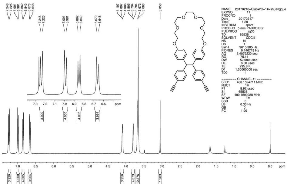
**Fig. S21.** <sup>1</sup>H NMR spectrum of compound 7 in CDCl<sub>3</sub>.
