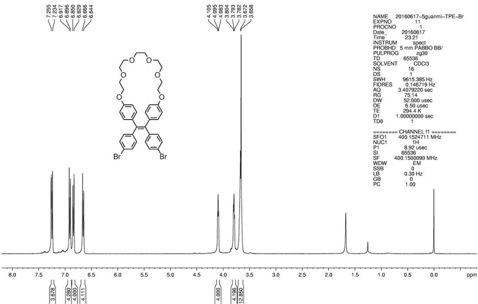
**Fig. S5.**  $^1\text{H}$  NMR spectrum of compound **3** in  $\text{CDCl}_3$ .
