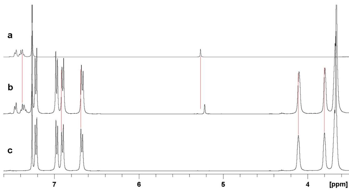
**Fig. S35.** <sup>1</sup>H NMR spectra of (R)-mandelic acid **9** (a), a mixture of (R)-**9** and macrocycle **6** (b) and macrocycle **6** (c) in  $\text{CDCl}_3$ .  $[\mathbf{9}] = [\mathbf{6}] = 5 \text{ mM}$ .
