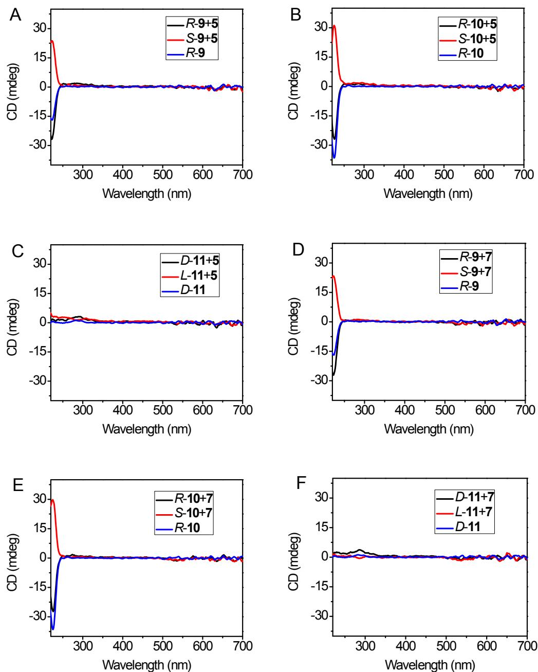
**Fig. S34.** CD spectra of a solution of intermediate **5** (A, B and C) and **7** (D, E and F) with enantiomer of chiral acid in 1,2-dichloroethane.  $[5] = [7] = 1/3[\text{chiral acid}] = 2.0 \times 10^{-4} \text{ M}$ .
