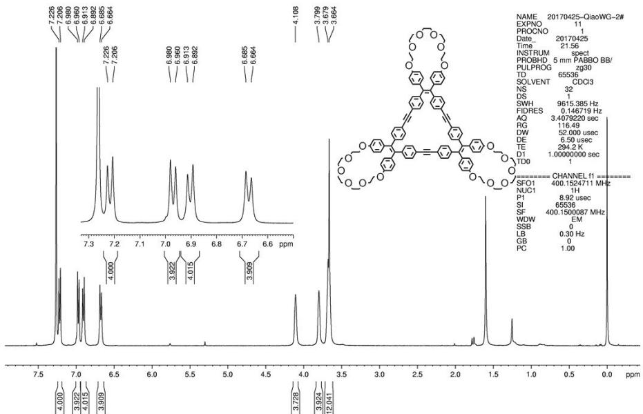
**Fig. S13.**  $^1\text{H}$  NMR spectrum of compound **6** in  $\text{CDCl}_3$ .
