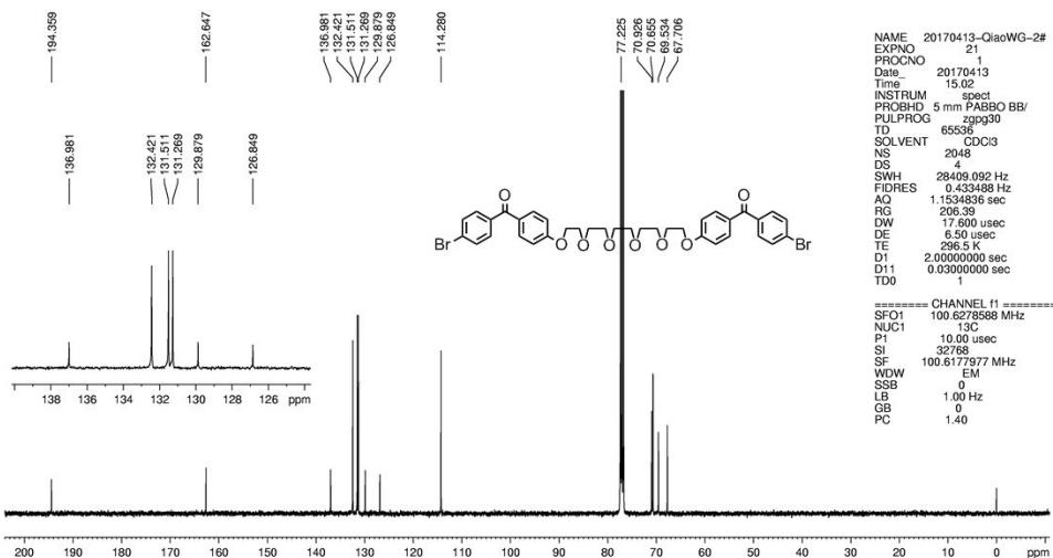
**Fig. S2.**  $^{13}\text{C}$  NMR spectrum of compound 2 in  $\text{CDCl}_3$ .
