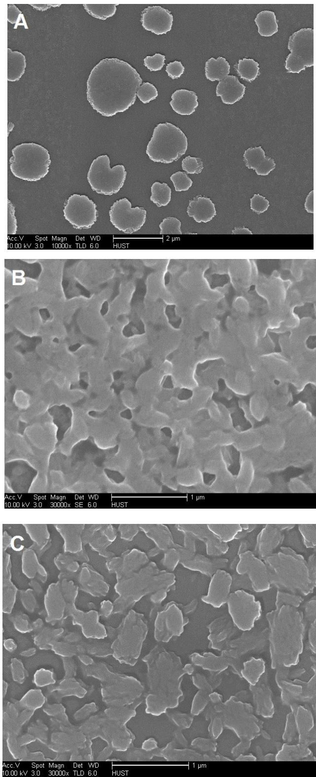
**Fig. S32.** FE-SEM images of film of **6** (A), **6-D-10** mixture and **6-L-10** mixture in 1,2-dichloroethane. The measurement sample was prepared by dropping the solution onto one glass slide and air dried.
