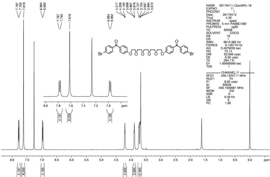
**Fig. S1.**  $^1\text{H}$  NMR spectrum of compound 2 in  $\text{CDCl}_3$ .
