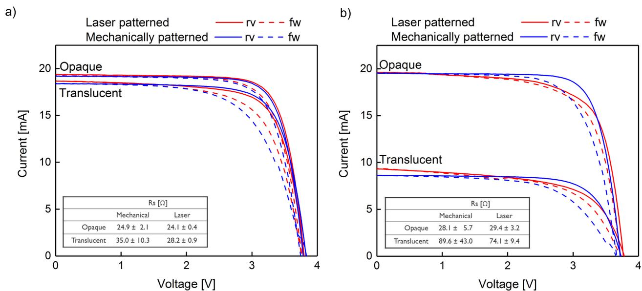
**Figure S 1** I-V curves of modules before (opaque) and after (translucent) partial area removal. The modules have been either laser (red) or mechanically (blue) patterned with a targeted transparent area ratio of a) 10 % and b) 50 %. Inset in each graph gives average  $R_s$  based on I-V scan for opaque and translucent modules.
