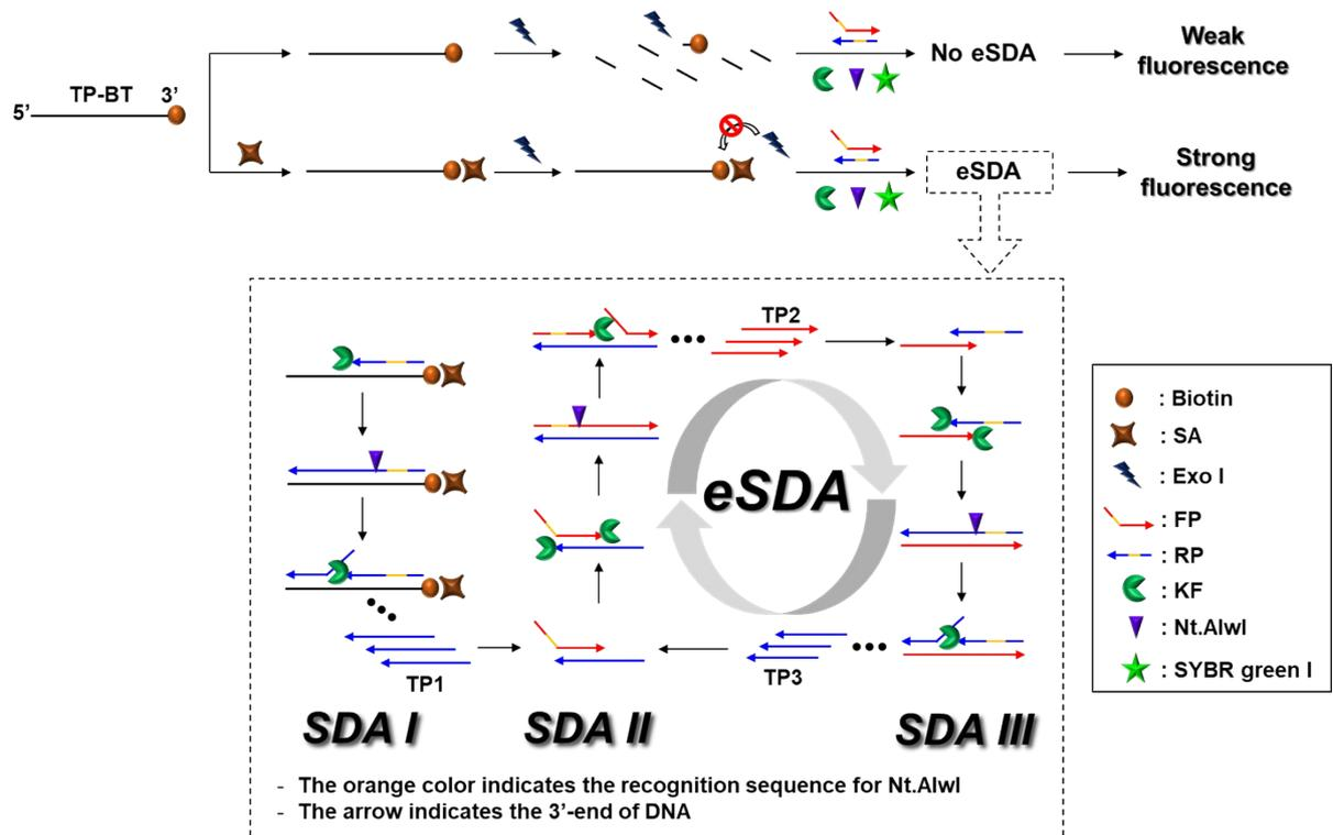
**Scheme 1** (Enlarged version) Schematic illustration of the detection strategy for biotin-SA interaction based on terminal protection-mediated eSDA.
