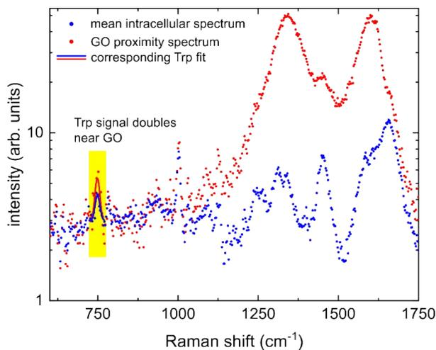
Figure S1 – The Raman spectra of the averaged intracellular matrix (blue) and the intracellular matrix in the proximity of GO flakes (red).
