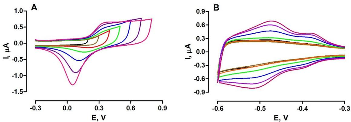
**Figure 1S:** (A) Effect of increasing oxidation potential on MO reduction peak and (B) subsequent H<sub>2</sub> peaks. Overlay of CVs performed over ranges between -0.65 V to +0.2/0.8 V vs. SCE at 100 mVsec<sup>-1</sup> in nitrogen (N<sub>2</sub>) saturated PBS (pH 7.4) at 25°C. Cycle 10 included for each CV.
