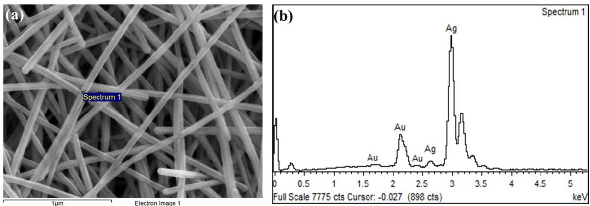
**Fig. S2.** Energy dispersive X-ray spectroscopy (EDS) of the 3D bimetallic 15 nm thick Au-coated Ag NWs structures. (a) An SEM image of 3D Au-Ag bimetallic NW structures. (b) Elemental analysis of the sample shows an Ag of 88.10% and an Au of 11.90%. The EDS data clearly confirms the 3D Au-Ag bimetallic NW structures.
