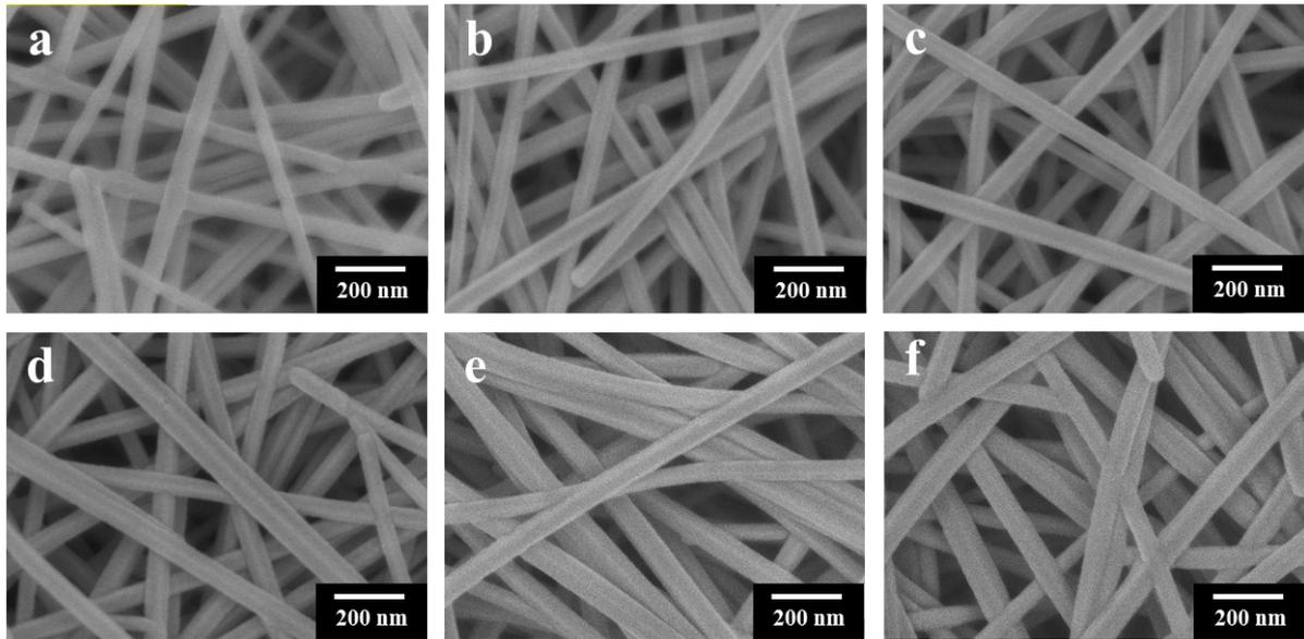
**Fig. S1.** Scanning electron microscopy (SEM) images of (a) the 3D stacked Ag nanowires (NWs) and 3D bimetallic (b) 5 nm, (c) 10 nm, (d) 15 nm, (e) 20 nm, (f) 25 nm thick Au-coated Ag NW structures.
