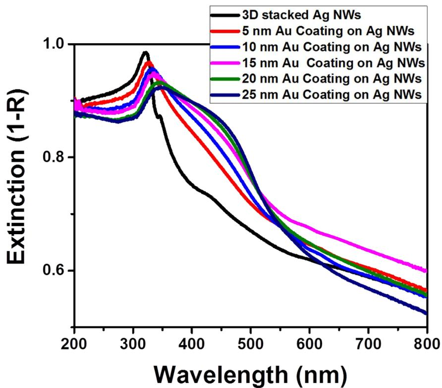
**Fig. S4.** Extinction spectra of the 3D Ag NW structures as a function of the Au deposition layer thickness.
