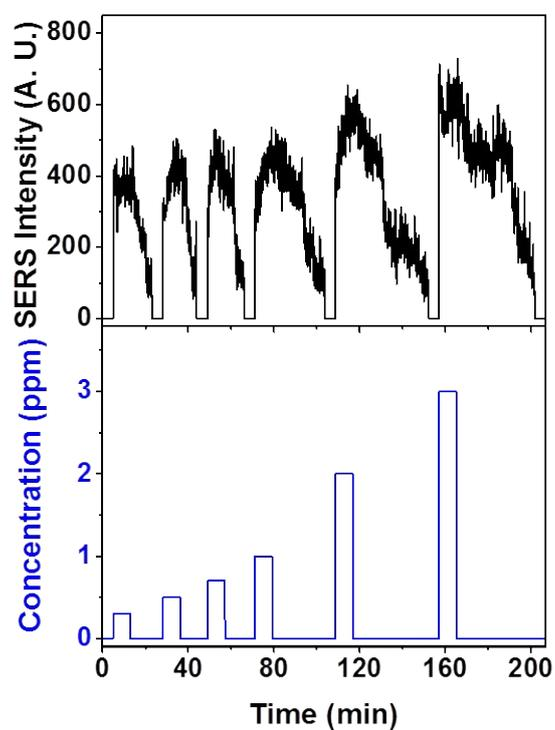
**Fig. S6.** Transient NO<sub>2</sub> gas response between 0.3 ppm and 3.0 ppm using the 3D hybrid Ag NW structures at RT.
