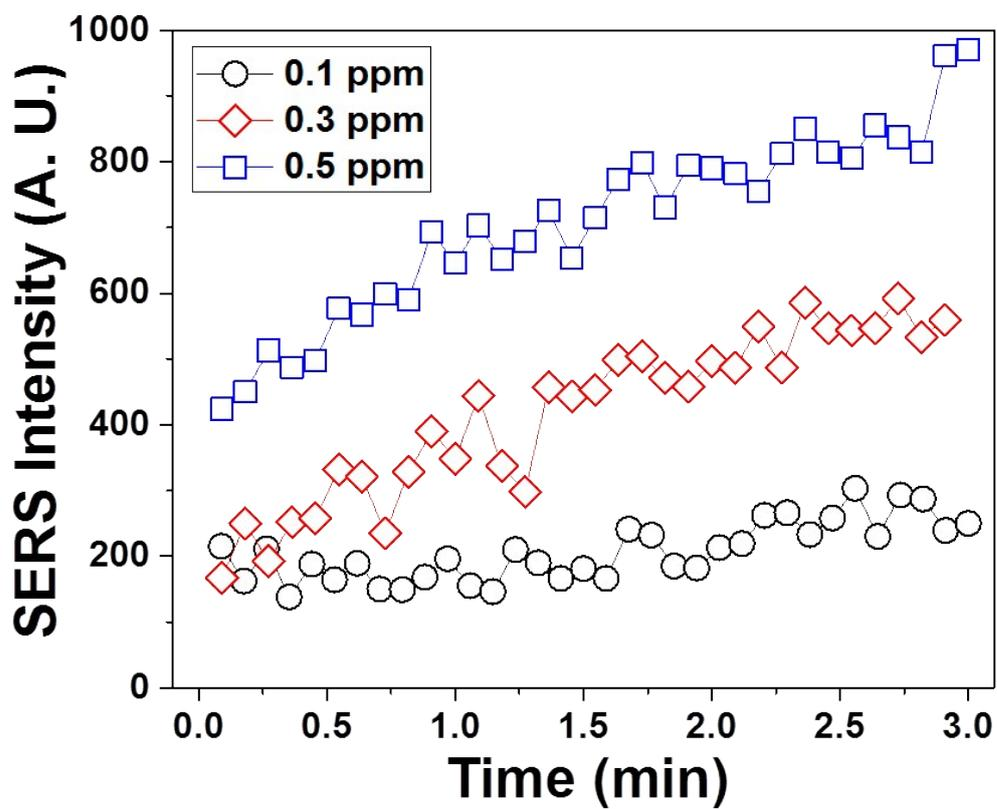
Fig. S5. SERS intensity changes at  $810\text{ cm}^{-1}$  as a function of the  $\text{NO}_2$  concentration.
