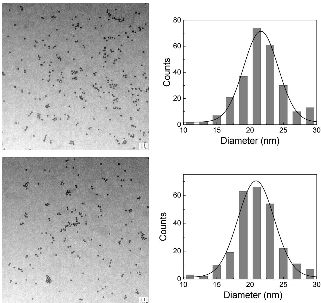
**Fig. S2** TEM images of MPA/MPS-AuNPs (top) and MUA/TEG-AuNPs (bottom) and respective size distribution histograms.
