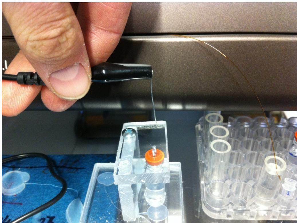
Figure S3. The process of putting the platinum electrode into the outlet vial containing electrophoretic buffer.
