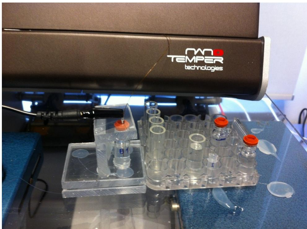
Figure S2. The outlet of the CE capillary inserted into the grounded vial.
