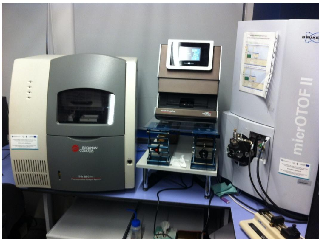
Figure S6. The CE, MST and MS instruments set in-line to visualize the potential triple on-line CE-MST-MS system.
