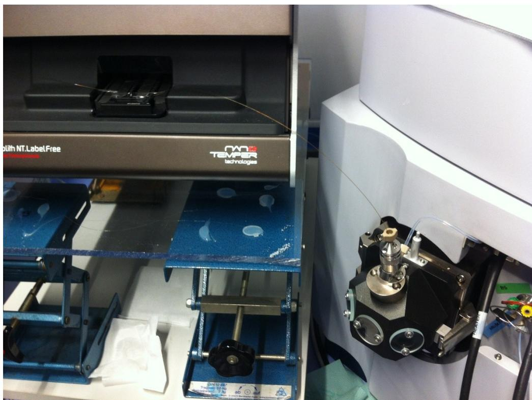
Figure S7. The outlet of the CE capillary (integrated with MST) inserted into the ion source of MS instrument (visualization of the potential new instrumentation/interface).
