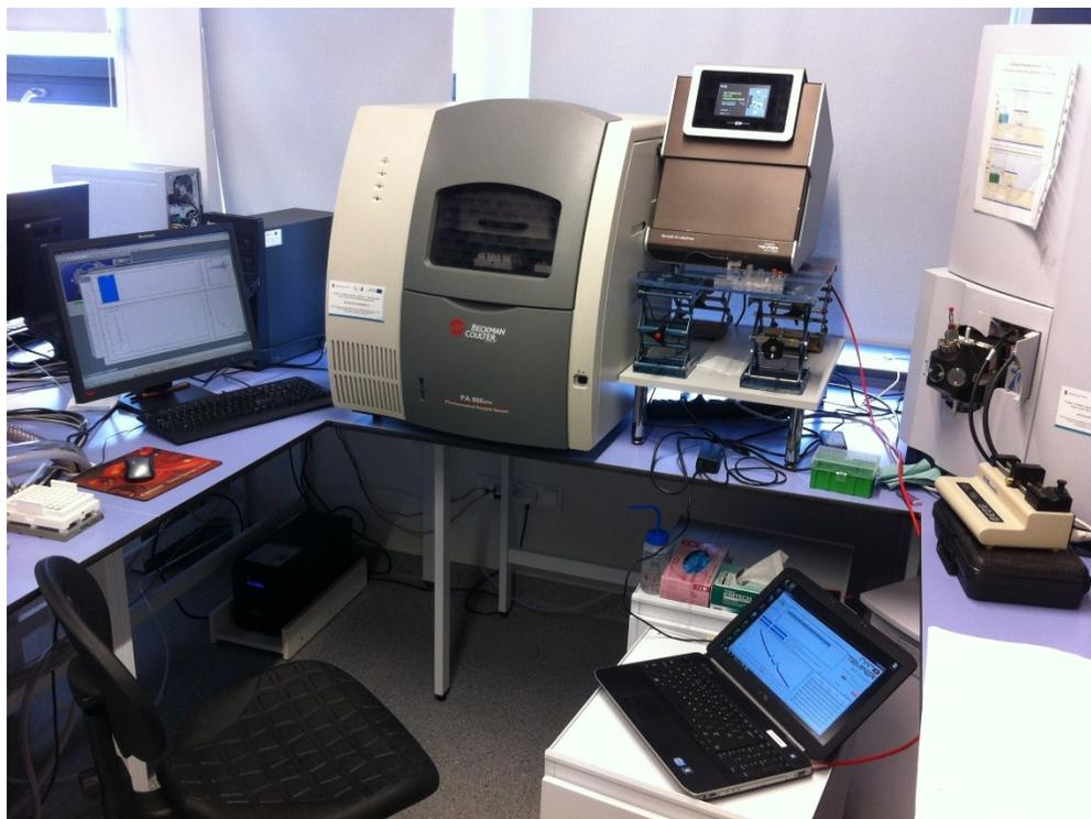
Figure S1. Photograph of the CE-MST instrumentation controlled by two distinct computers.
