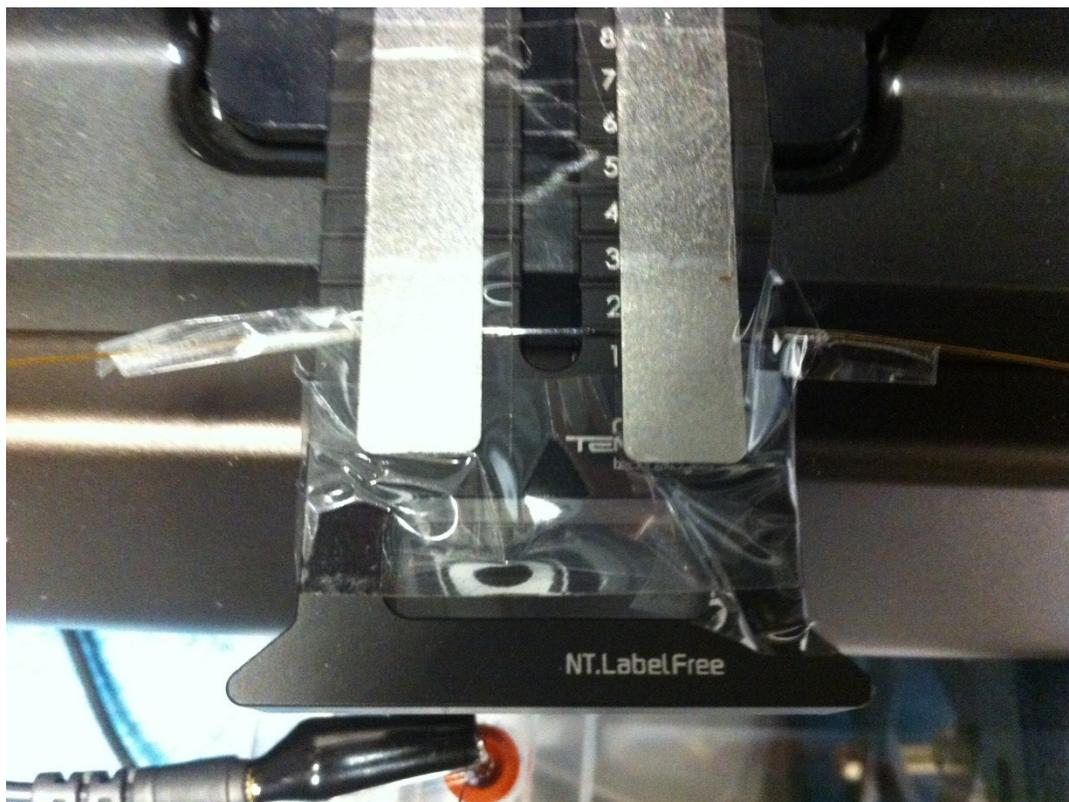
Figure S5. The “capillary-in-capillary” interface. The capillary position was stabilized by using sticky tape. In the middle part the CE capillary was transparent (the coating was burned off).
