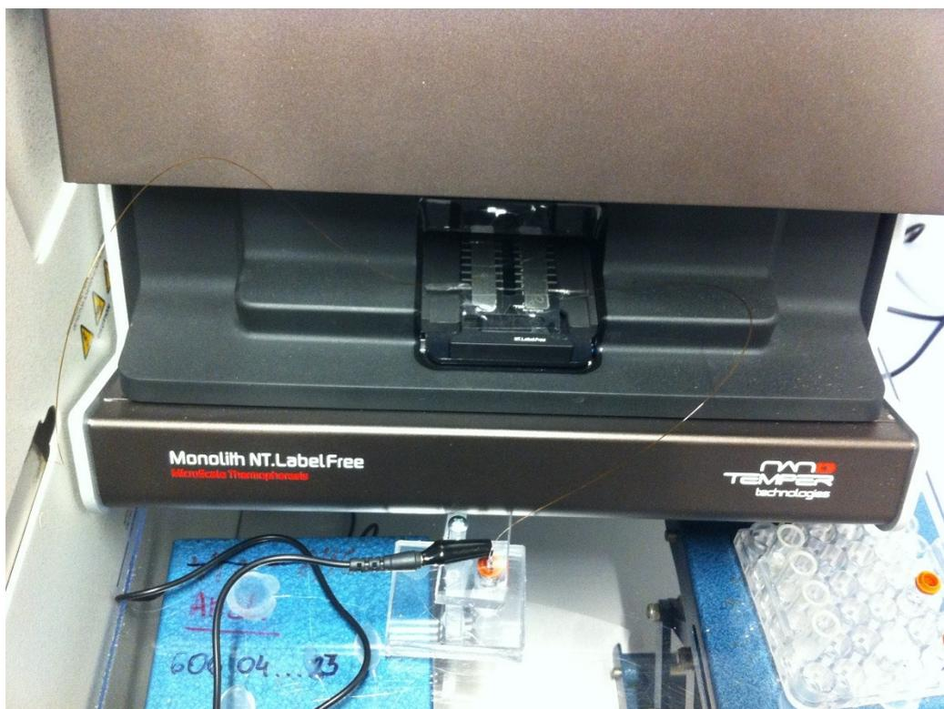
Figure S4. The CE capillary brought out the CE instrument, mounted onto the MST tray/table inside the MST capillary (MST instrument was opened to show interior).
