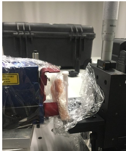
Figure S4 – Experimental set up involving the tracking of nanotags through tissue. The nanotags were held in a microcuvette and obscured by the tissue. The point and shoot adaptor was used to bring the tissue into contact with the instrument, thus ensuring there was no space between the tissue and the instrument.
