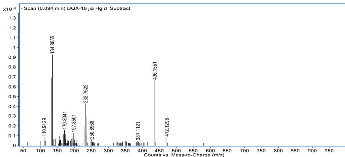
**Figure S7.** The HRMS of reaction products of probe and  $\text{Hg}^{2+}$
