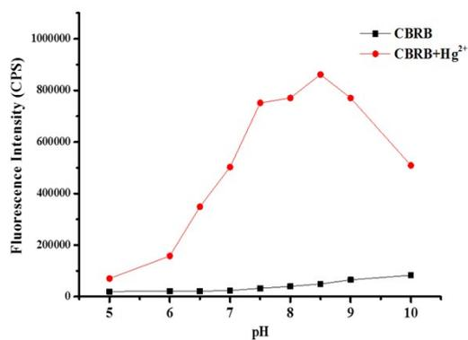
**Figure S3.** Fluorescence responses (625 nm) of probe **CBRB** (5  $\mu\text{M}$ ) and after addition of 5  $\mu\text{M}$   $\text{Hg}^{2+}$  in 5 mM HEPES aqueous solution as a function of different pH values.
