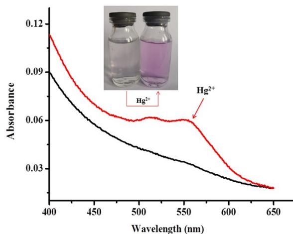
**Figure S1.** Absorption spectra of probe **CBRB** (20  $\mu\text{M}$ ) upon addition of  $\text{Hg}^{2+}$  (20  $\mu\text{M}$ ) in 5 mM HEPES (pH 7.4) aqueous solution. The illustration shows the change of color for adding  $\text{Hg}^{2+}$  to probe **CBRB**.
