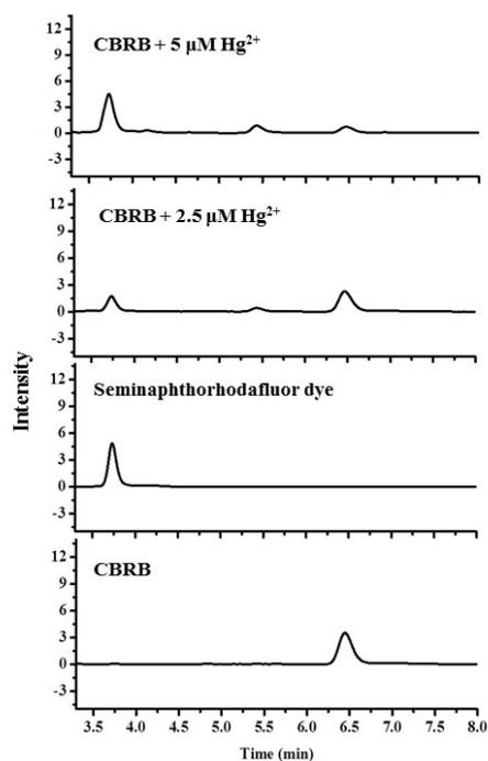
**Figure S8.** HPLC chromatogram traces of probe **CBRB** before or after the treatment of  $\text{Hg}^{2+}$  for 20 min. The peak corresponding to **CBRB** decreased in an  $\text{Hg}^{2+}$ -dose independent way accompanied by the simultaneous increase of a new peak whose structure was elucidated by HRMS analysis to be the seminaphthorhodafuor dye.
