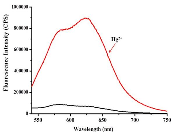
**Figure S2.** Fluorescence spectra of probe **CBRB** (5  $\mu\text{M}$ ) in the presence of 5  $\mu\text{M}$   $\text{Hg}^{2+}$  under aqueous solution containing 5 mM HEPES (pH 7.4).
