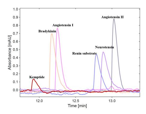
Figure S4. Six overlapped UV records of tCITP separations of individual peptide solution including Kemptide, bradykinin, angiotensin I, renin substrate, neurotensin and angiotensin II at  $2~\mu M$  concentration
