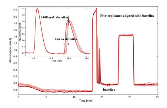
Figure S2. UV records from five replicates of tCITP separation for two peptides in 2  $\mu$ M sample concentration and at 45% sample loading
