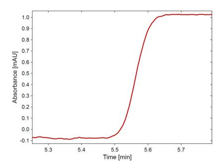
Figure S1. Sample flow rate measurement at 5 psi nitrogen pressure
