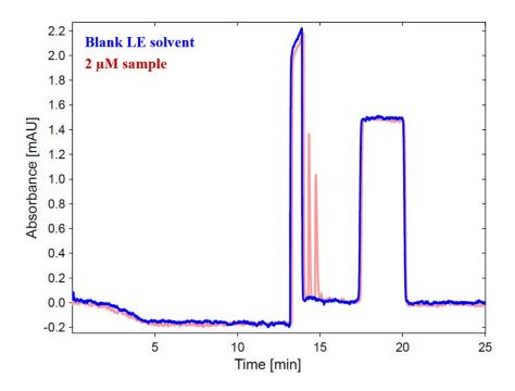
Figure S3. Comparison of the UV records from tCITP separations of the two peptides in 2  $\mu\text{M}$  concentration and blank LE solvent
