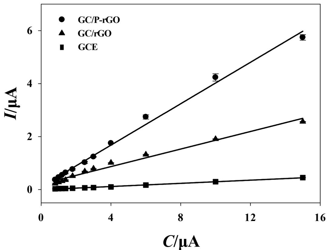
Fig. S3 Current values vs DA concentration of different modified electrode by LSV (mean  $\pm$  SD, n=3).
