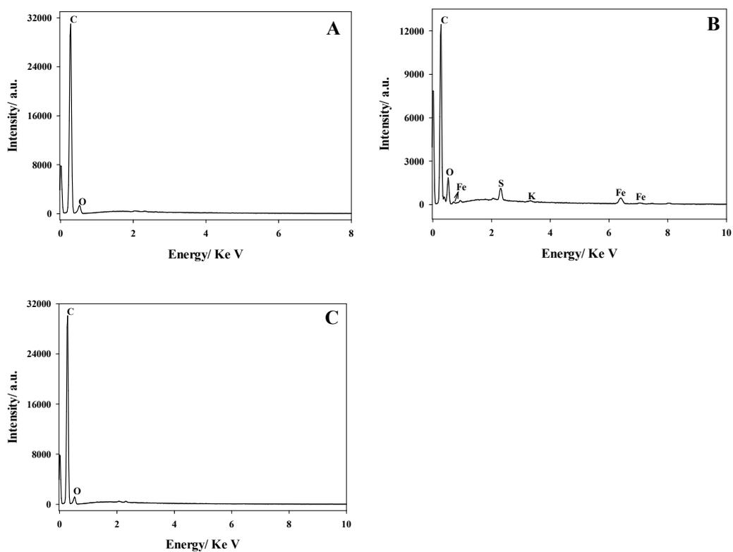
Fig. S2 EDX spectrum of bare GC (A), rGO@PB (b), P-rGO(C)
