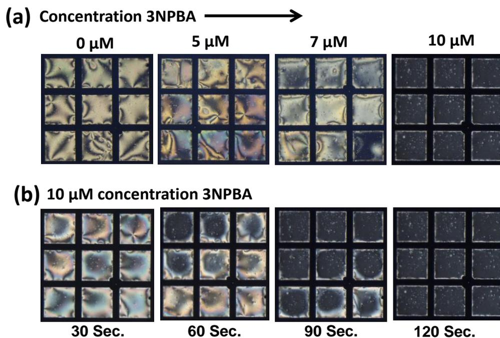
**Figure S1.** (a) Cross-polarized optical images of 5CB when exposed to different concentrations of 3NPBA aqueous solution. Images are taken after 5 min of stabilization of LC-aqueous interface. (b) Time lapse orientation transition of 5CB from planar (bright image) to homeotropic (black image) in contact with 10  $\mu\text{M}$  of 3NPBA aqueous solution (282  $\mu\text{m}$  square grid size; 20  $\mu\text{m}$  depth).
