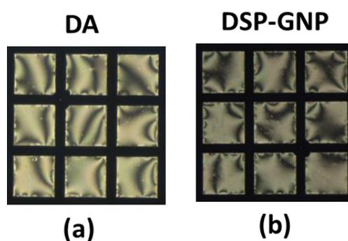
**Figure S2.** POM images of 5CB at LC-aqueous interface in contact with (a) dopamine of 1 mM concentration and (b) 0.17 nM concentration of DSP-GNPs. The images are taken after 20 minutes of stabilization of LC-aqueous interface (282  $\mu\text{m}$  square grid size; 20  $\mu\text{m}$  depth).
