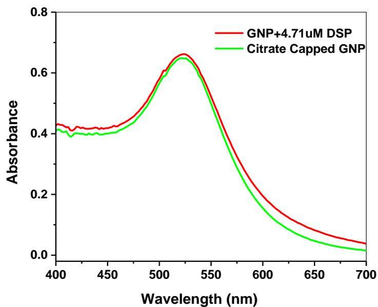
**Figure S3.** UV-Vis absorption spectra of 13 nm diameter GNPs (green) and DSP functionalized GNPs (DSP-GNPs) (red). The concentration of the GNPs were determined from its absorbance ( $\epsilon = 2.7 \times 10^8 \text{ M}^{-1} \text{ cm}^{-1}$  at  $\lambda=520 \text{ nm}$ ).
