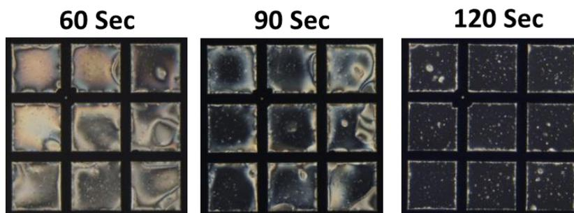
**Figure S4.** Time lapse orientational transition of 5CB from planar (bright image) to homeotropic (black image) in contact with  $10 \mu\text{M}$  of 3NPBA and  $0.17 \text{ nM}$  of DSP-GNP aqueous solution ( $282 \mu\text{m}$  square grid size;  $20 \mu\text{m}$  depth).
