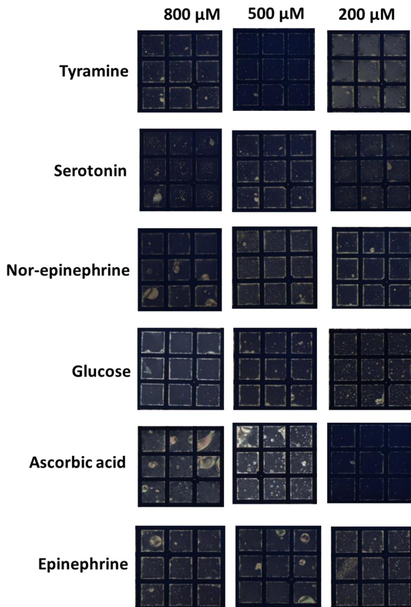
**Figure S9.** POM images of 5CB at LC-aqueous interface in contact with 0.17 nM concentration of DSP-GNPs and 10  $\mu\text{M}$  of 3NPBA with different structurally similar molecules at different concentrations (282  $\mu\text{m}$  square grid size; 20  $\mu\text{m}$  depth). The images are taken after 20 minutes of stabilization of LC-aqueous interface.
