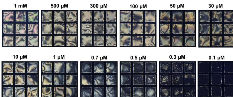
**Figure S6.** Polarized image of LCs immersed in the aqueous solution containing different concentration of dopamine with 10 μM of 3NPBA and 0.17 nM of DSP-GNP (282 μm square grid size; 20 μm depth). The images are taken after 20 minutes of stabilization of LC-aqueous interface.
