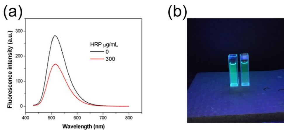
**Fig. S9.** (a) The Fluorescence spectra of synthesized CNDs before and after the addition of 300  $\mu\text{g/mL}$  HRP. (b) The images of CND solution before (left) and after (right) the addition of 300  $\mu\text{g/mL}$  HRP under 365 nm ultraviolet light.
