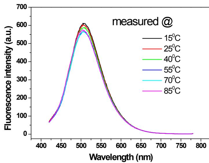
**Fig. S5.** Fluorescence spectra of synthesized CNDs at various temperatures.
