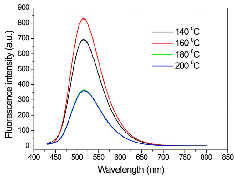
**Fig. S2.** Fluorescence spectra of CNDs synthesized at different temperatures.
