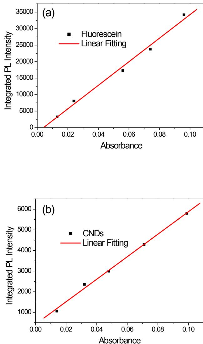
**Fig. S3.** Plots of the integrated PL intensity of (a) fluorescein in 0.1 M NaOH, and (b) boronic acid-functionalized CNDs in water as a function of optical absorbance at 410 nm.
