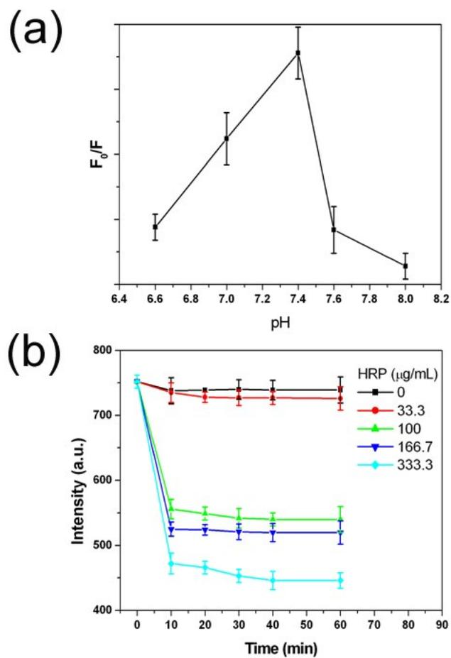
**Fig. S7.** (a) Effects of pH on the detection of HRP.  $F_0$  and  $F$  represent the fluorescence intensities of CNDs at 514 nm in the absence and presence of HRP, respectively. HRP concentration: 333.3  $\mu\text{g/mL}$ . (b) Effects of incubation time on the fluorescence intensities of the CND system.
