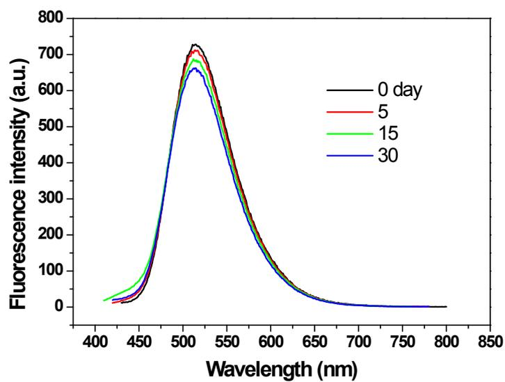
**Fig. S6.** Fluorescence spectra of synthesized CNDs after different periods of storage.
