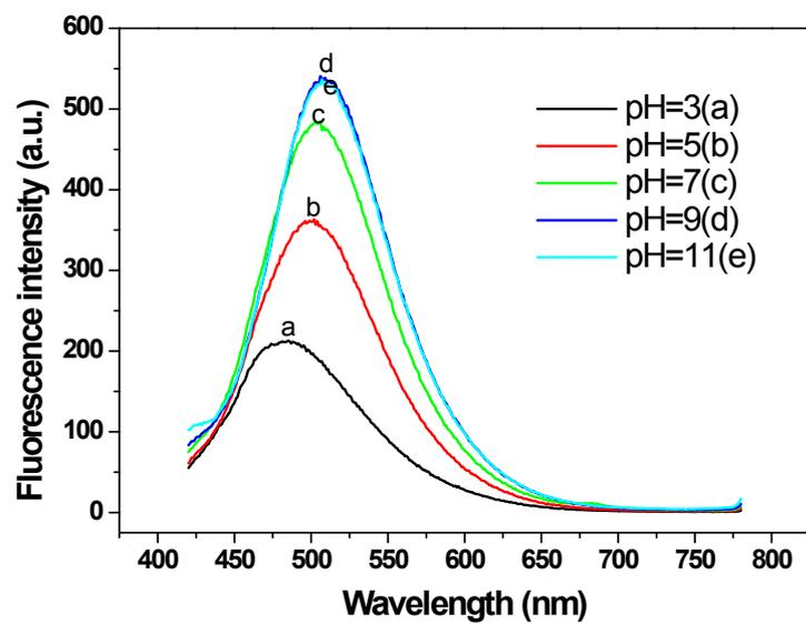
**Fig. S8.** Fluorescence spectra of synthesized CNDs in 10 mM phosphate buffer solutions of various pH values ranging from 3 to 11.
