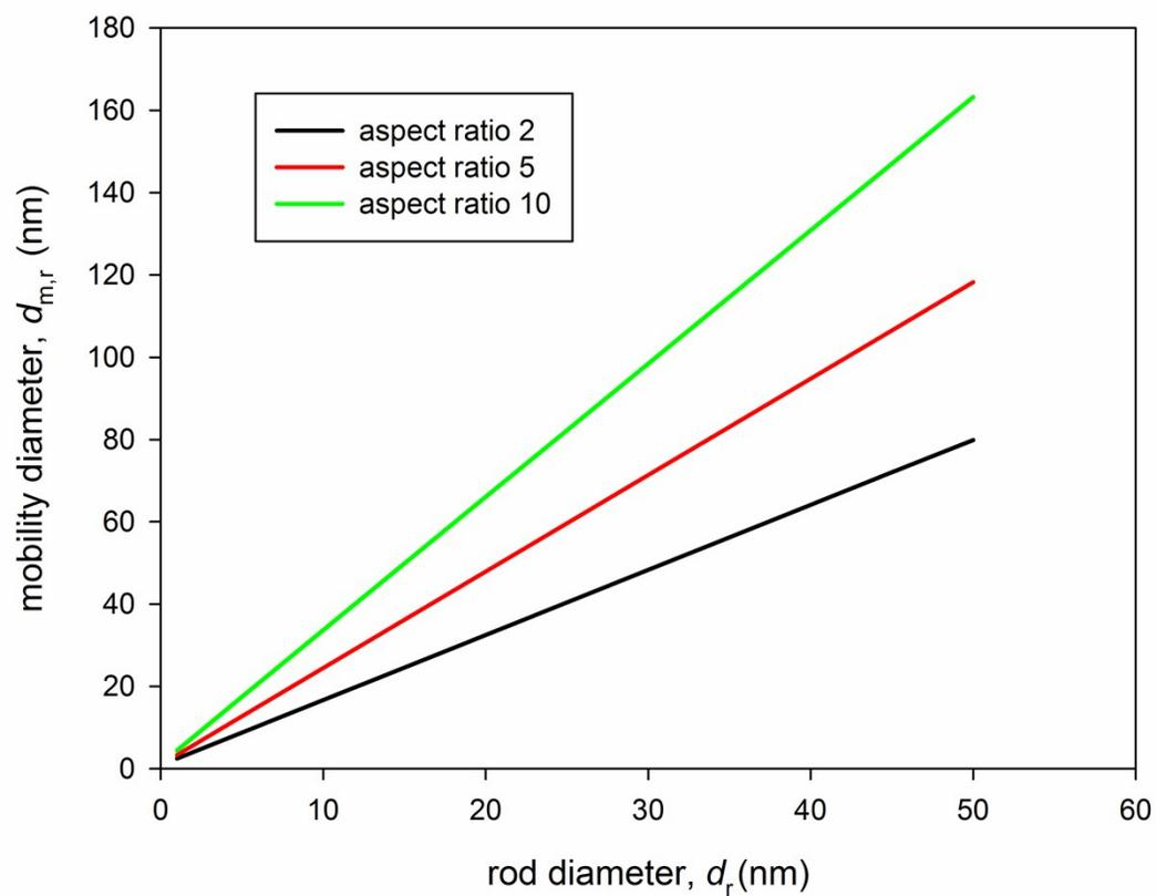
Figure S1. Graphical presentation of Eq. (1) showing the relationship between mobility diameter and rod (cylindrical) diameter as a function of aspect ratio ( $L_r/d_r$ ) for model rods.  $\Delta d_{gas} = 0.68$  nm.
