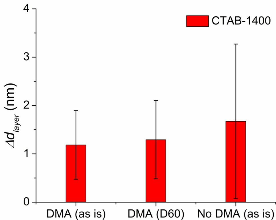
Figure S3. Measurement of adlayer thickness showing the effect of dilution and collection method. D60 indicates 60× dilution compared with the native suspension. The adlayer thickness observed with DMA size selection is compared with that without DMA selection. Neither the effect of dilution nor DMA selection has an obvious effect on adlayer thickness. Roughly 10 GNRs and multiple locations along each GNR were measured to yield an average and one standard deviation.
