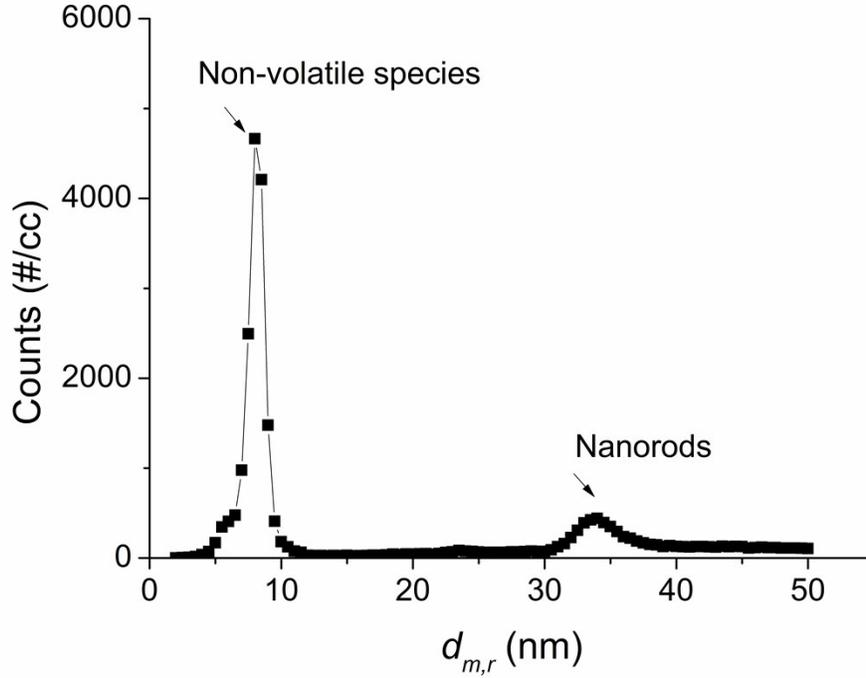
Figure S5. Contribution of non-volatiles from ES to the adlayer thickness. Mobility size distribution of CIT-600 by ES-DMA-CPC (CPC is a condensation particle counter).
