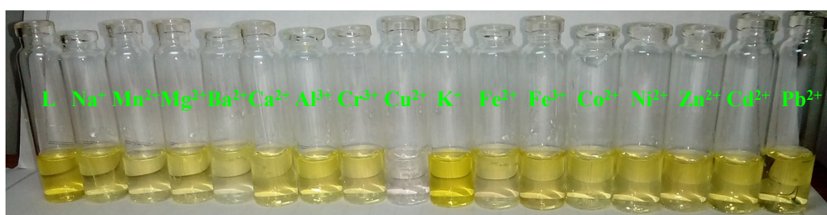
Fig. S8. The colour changes of L (10 μM) upon addition of various cations (10 equiv.) in MeCN-H 2 O (2:1, v/v) at room temperature.
