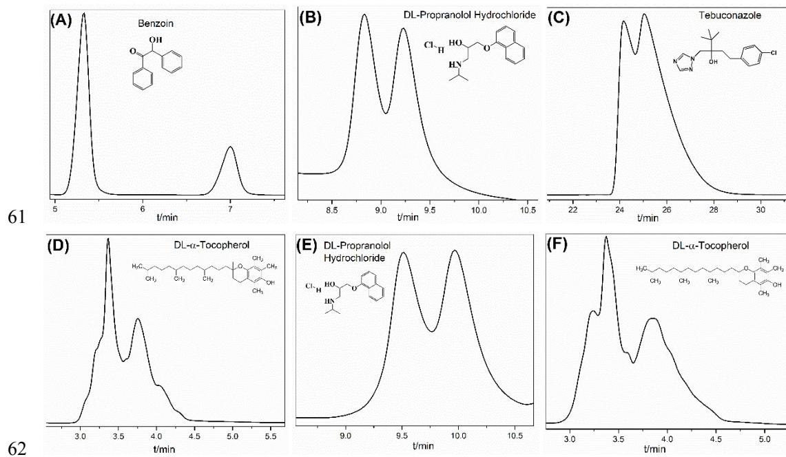
63 **Figure S6.** Chromatographic resolution of some chiral drug and pesticide molecules on HPLC
