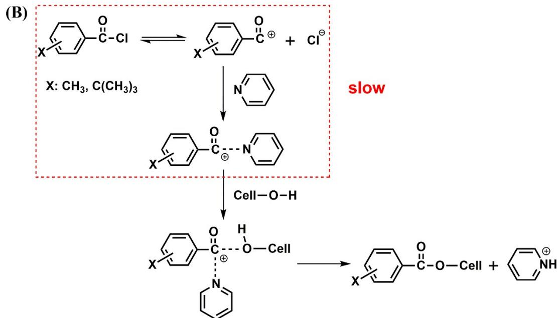
17 **Figure S1.** The possible mechanism of homogeneous benzoylation of cellulose with pyridine as the
