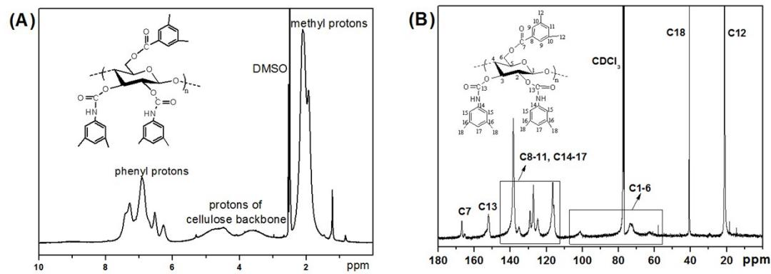
55 **Figure S4.** (A)  $^1\text{H-NMR}$  and (B)  $^{13}\text{C-NMR}$  spectra of cellulose 3,5-dimethylbenzoate 3,5-dimethyl
