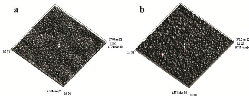
Fig. S1 AFM images of the GCE/CS-SCS- $\alpha$ -CD (a) surfaces and of the GCE/CS-SCS- $\gamma$ -CD surface.
