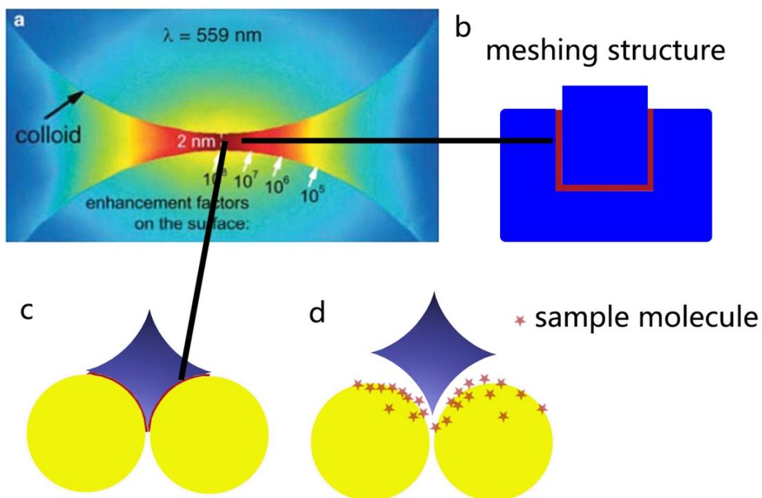
Fig. S10 Enhancement factor distribution in a hot spot formed between two gold nanoparticles separated by 2 nm plotted on a logarithmic scale (a).<sup>1</sup> Scheme illustration of SERS hot-spots of meshing structure (b), tip-gap meshing structure. Detection schematic diagram of the protocol we proposed (d).
