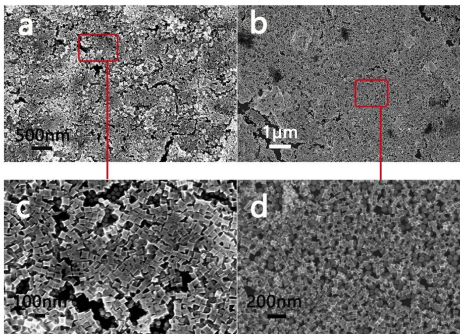
Fig. S6 SEM images of (a and c) “non-meshing” bilayer, substrates, b and d “tip-gap” bilayer substrate.
