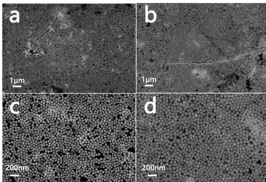
Fig. S7 SEM images of (a and c), Au NSs monolayer before dropping sample, (b and d) after dropping sample.
