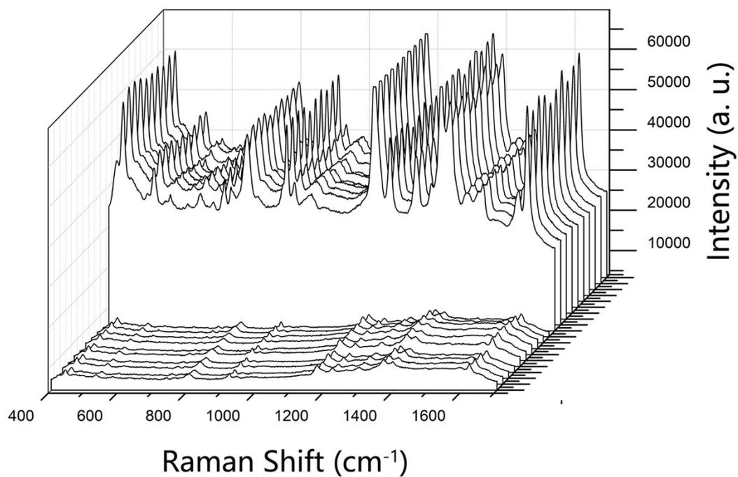
Fig. S8 SERS spectra of  $10^{-7}$  and  $10^{-11}$  M MG collected from ten different positions on the tip-gap meshing SERS substrate.
