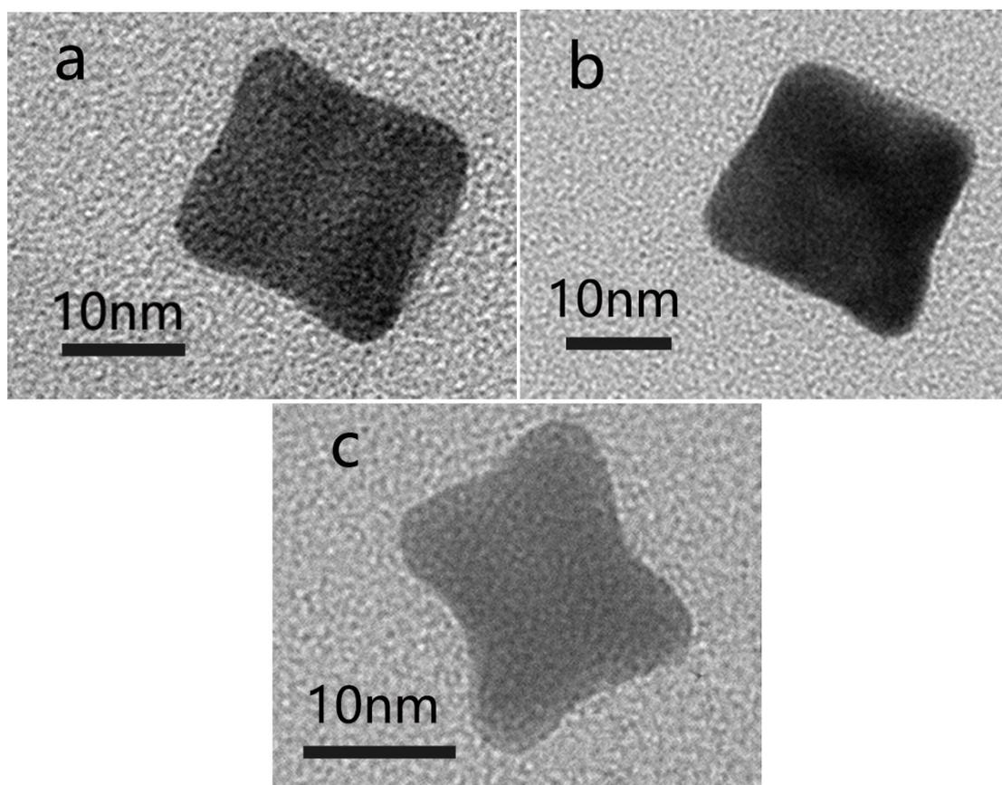
Fig. S2 TEM images of intermediate products of the CENCs, reaction for 30 min (a), 90 min (b), 120 min (c).
