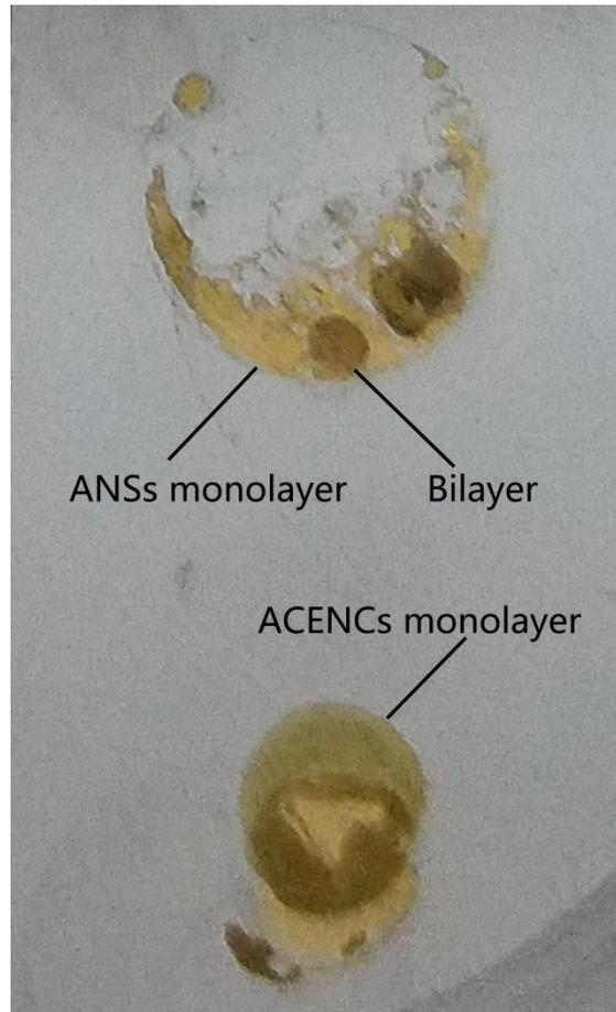
Fig. S5 Images of CENCs monolayer, Au NSs monolayer and bilayer substrate
