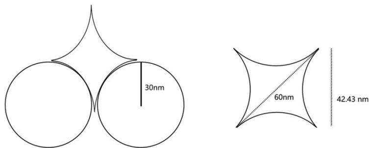
Fig. S4 Geometric calculation of the size of CENCs in condition of 60nm
