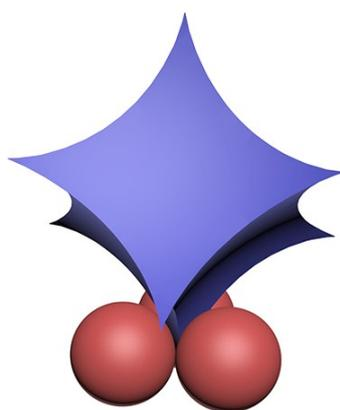
Fig. S9 Depict of the tip-gap meshing structure when the size of CENCs is much bigger than Au NSs.
