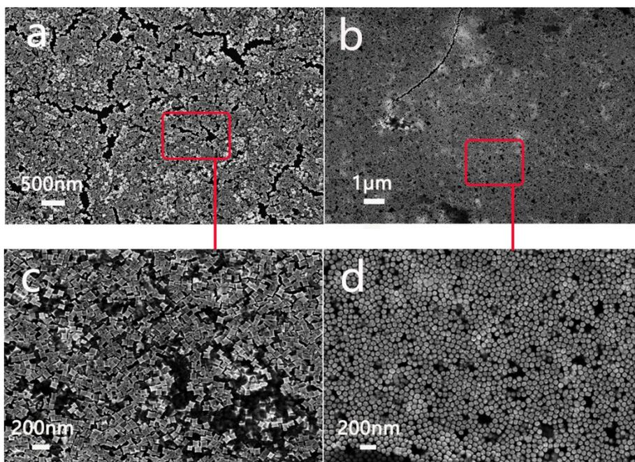
Fig. S3 SEM images of (a and c), CENCs monolayer, (b and d) Au NSs monolayer.
