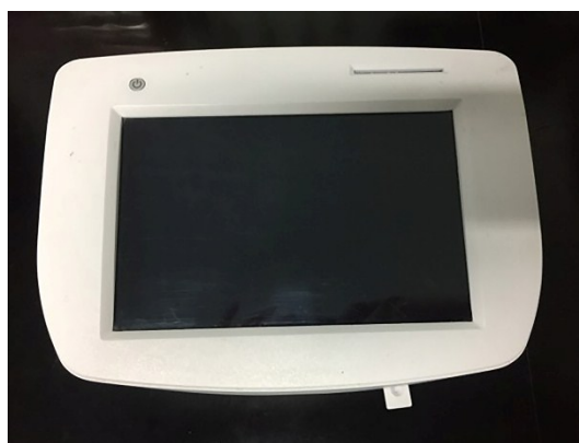
Fig. S1 Portable test strip reader with touch screen integrated with test strip in the test tray
