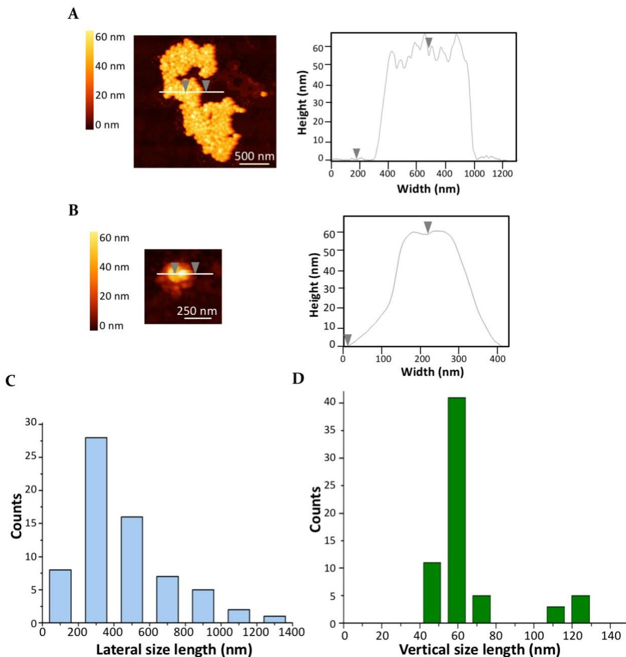
**Figure S4.** AFM characterization of: (A) A representative AgNPs aggregate on glass (left) with the section analysis along the line marked in the image (right); (B) A typical AgNPs aggregate in presence of alizarin ( $10^{-5}$  M) on glass with the relative section analysis. (C) Lateral size and (D) height distribution of AgNPs aggregates in presence of alizarin (about 65 measured aggregates from 100 inkjetted droplets).
