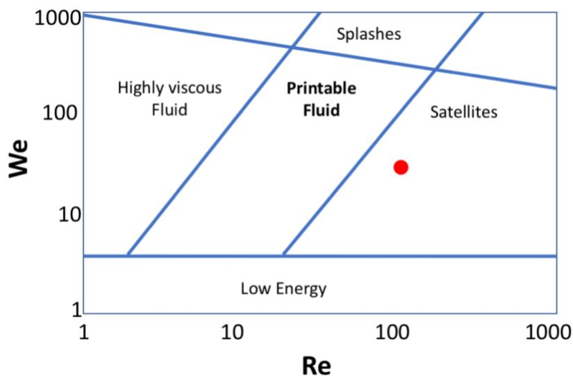
**Figure S2.** Collocation of the employed aqueous inks (red dot) within the Derby plot which illustrates the different regimens of inkjet printing. It is clear to observe that our ink represents a classical example of a fluid which would easily form satellites.
