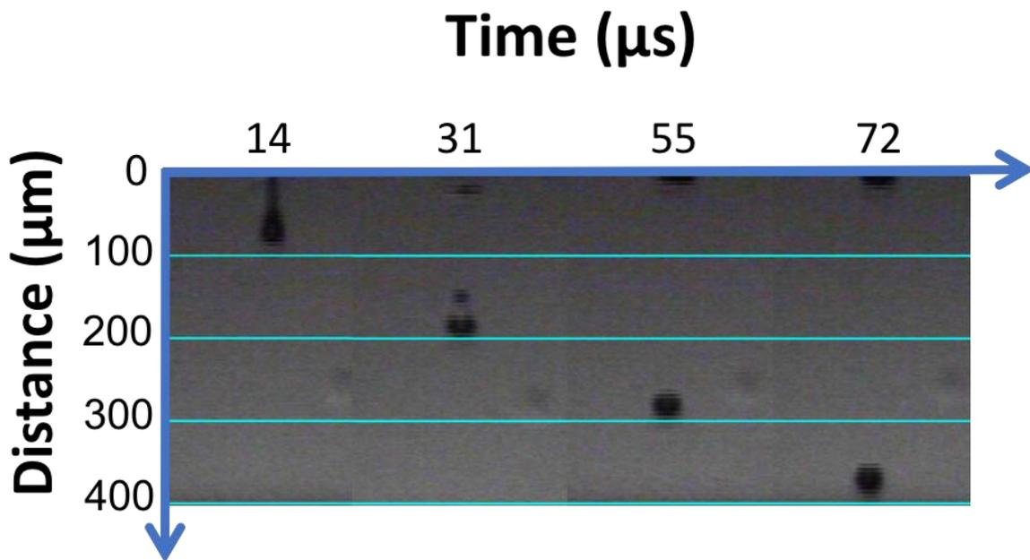
**Figure S3.** Stroboscopic images of 10 pL (nominal volume) droplets formation of an ink containing Ag NPs (1:10) and alizarin ( $10^{-5}$ M). The stroboscopic pictures are captured while a droplet pinches-off at nozzle exit (14  $\mu$ s). Satellite recoil occurs after 55  $\mu$ s, leading to reproducible production of spherical droplets without satellites.
