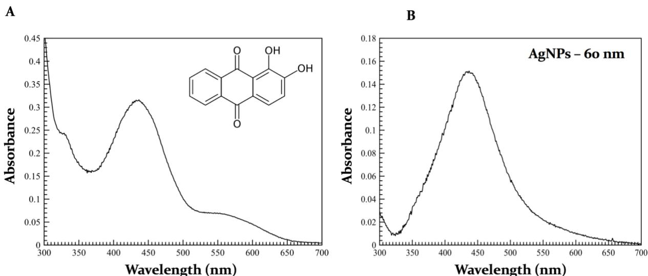
**Figure S1.** (A). UV-vis spectra of Alizarin 10<sup>-4</sup> M in ethanol and (B) Ag NPs 60 nm diluted 1:10 in water.
