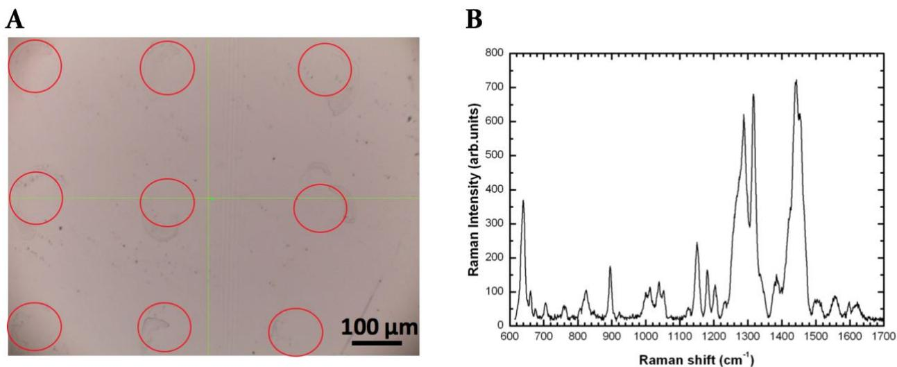
**Figure S5.** (A) Optical image of 9 dried droplets (marked by red circles) containing Ag NPs (1:10) and alizarin ( $10^{-5}$ M) at 1000 pL level, and (B) relative SERS spectra from a single hot spot.
