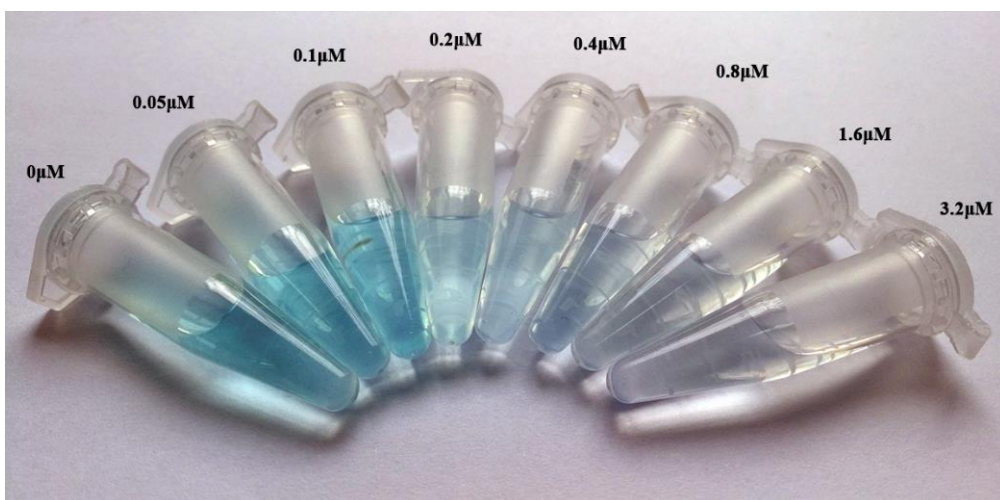
Fig.S1 Photograph of NBA in the presence of various concentrations of PFOS from 0 \mu\text{mol/L} to 3.2 \mu\text{mol/L} ; NBA, 0.3 \mu\text{mol/L} ; pH, 3.3.
