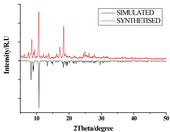
**Figure S2.** The experimental powder X-ray diffractogram of as-synthesised ZnBND (normal plot) and corresponding simulation result (inverted plot).
