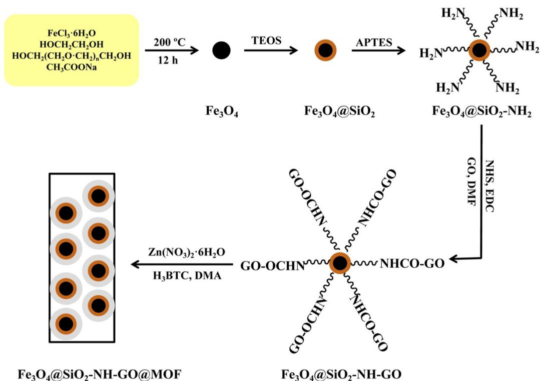
**Figure S1.** Preparation of  $\text{Fe}_3\text{O}_4@\text{SiO}_2\text{-NH}_2@\text{ZnBND}$ (MGO-ZnBND)
