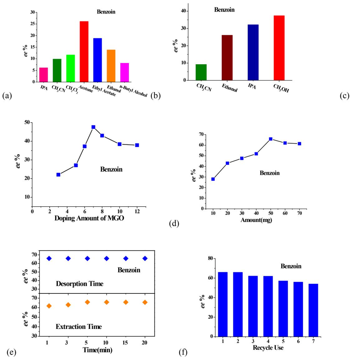
**Figure S3.** “Enantioselective capture” process for benzoin using MGO-ZnBND. (a) Optimization of the extraction solvent; (b) Optimization of the elution solvent; (c) Optimization of the percentage of MGO; (d) Optimization of the dosage of MGO-ZnBND; (e) Optimization of the extraction time and desorption time; (f) Recycle use of MGO-ZnBND composite.
