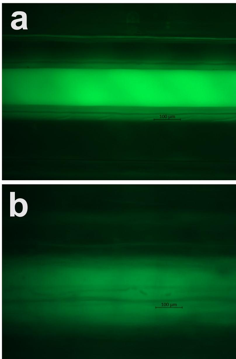
Figure SI2 – a) Fluorescence optical image obtained from a channel made of PLA and PMMA by the proposed method filled with  $100 \mu\text{mol L}^{-1}$  fluorescein. b) Fluorescence optical image of a microchannel made completely from PLA filled with the same solution. Scale bars are  $100 \mu\text{m}$ .
