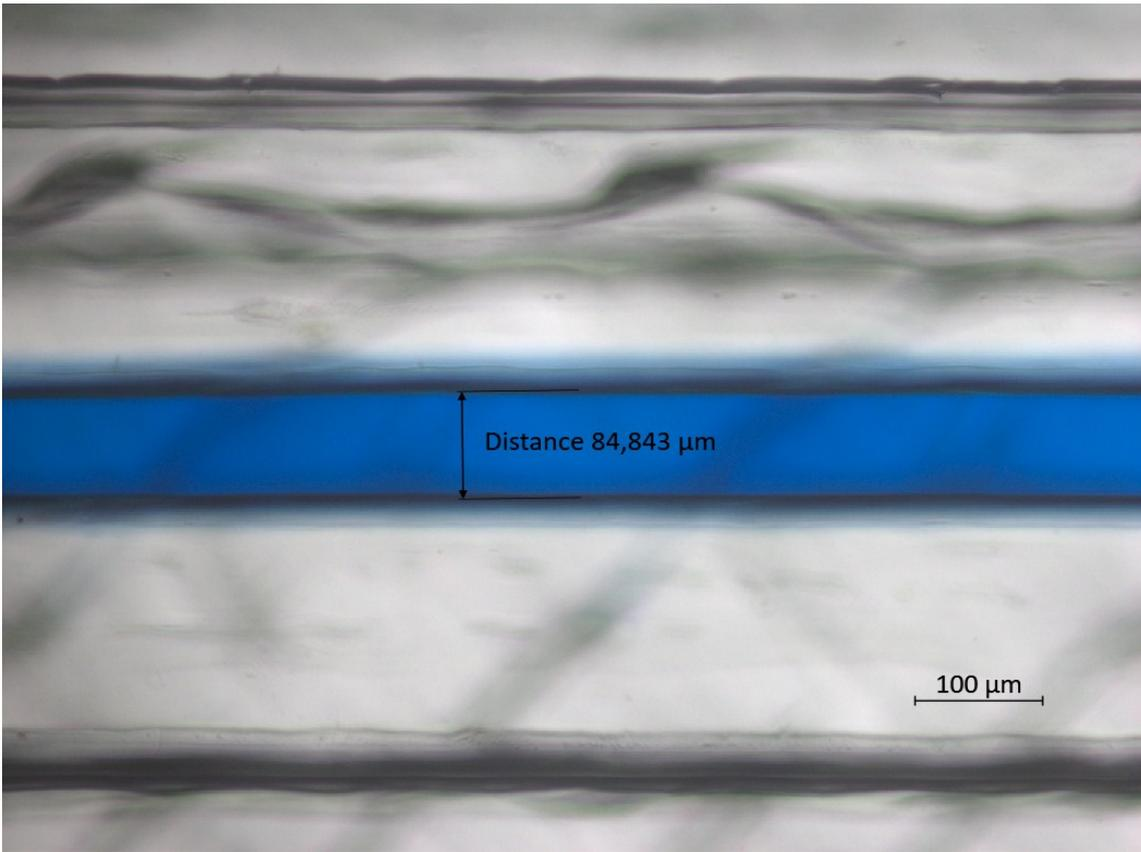
Figure SI3 – Optical image of a channel created by the proposed protocol with 85  $\mu\text{m}$  width. The channel was filled with blue colorant.
