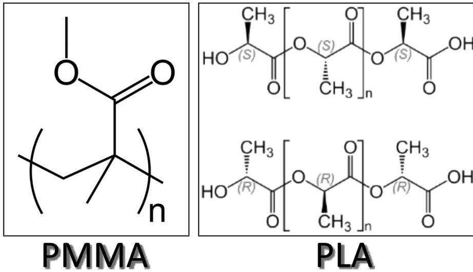
Figure SI1 – Chemical Structure of poly(methyl methacrylate) (PMMA) and poly(lactic acid) (PLA)
