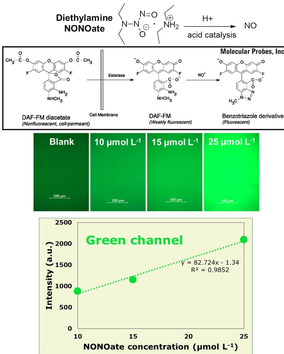
Figure SI7 – Nitric oxide measurement in the device from Figure SI4. Three different concentrations (10 to 25  $\mu\text{mol L}^{-1}$ ) of nitric oxide were measured from NONOate precursor. The scale bars are 100  $\mu\text{m}$ .
