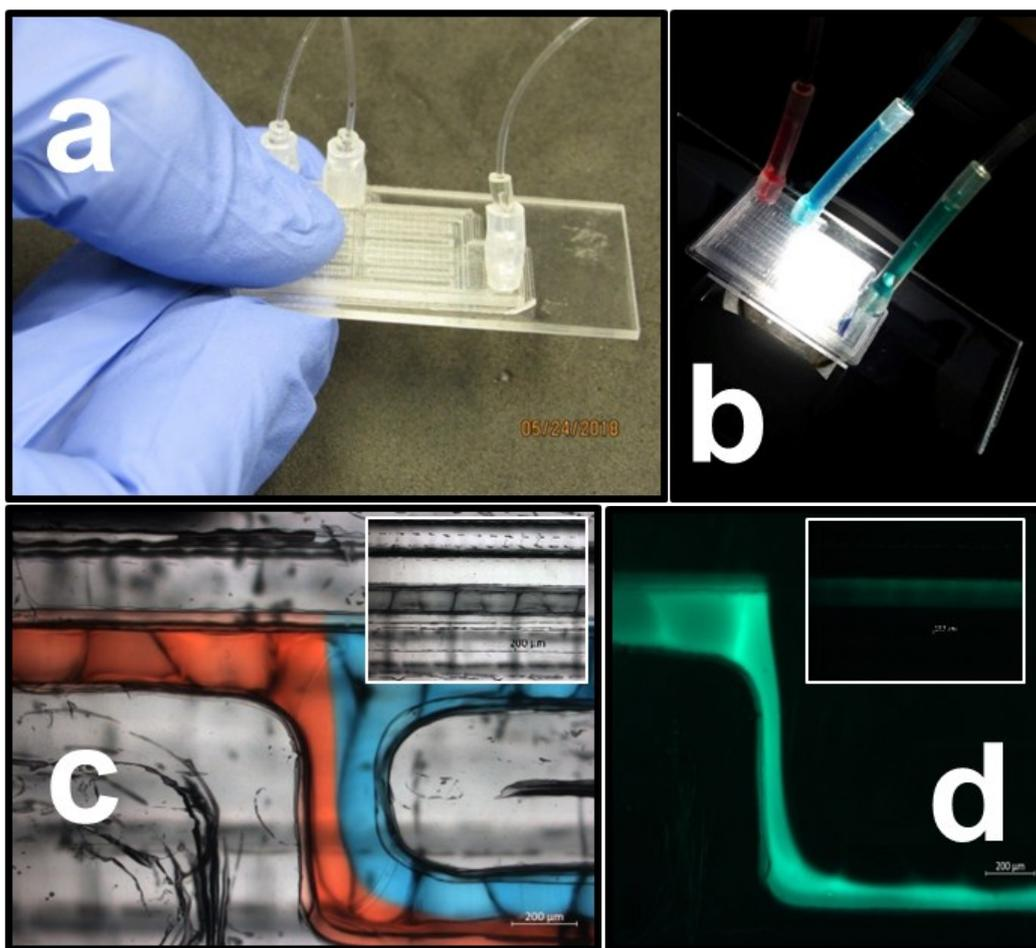
Figure SI4 – a) Photograph of the final device. b) Microfluidic mixer mounted over on the inverted microscope. c) Zoom of the confluence region (food dyes were used for contrast purposes) where the inset shows the two fluids fully mixed. d) Fluorescence photograph of the confluence region (a  $100 \mu\text{mol L}^{-1}$  fluorescein solution was used) where the inset shows the two fluids fully mixed.
