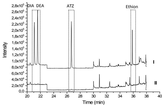
**Figure S4.** Chromatogram in: I) matrix fortified with ATZ, DEA ( $2.0\mu\text{g L}^{-1}$ ) and DIA ( $3.0\mu\text{g L}^{-1}$ ) and Ethion ( $2.0\mu\text{g L}^{-1}$ ). II) non-fortified matrix.
