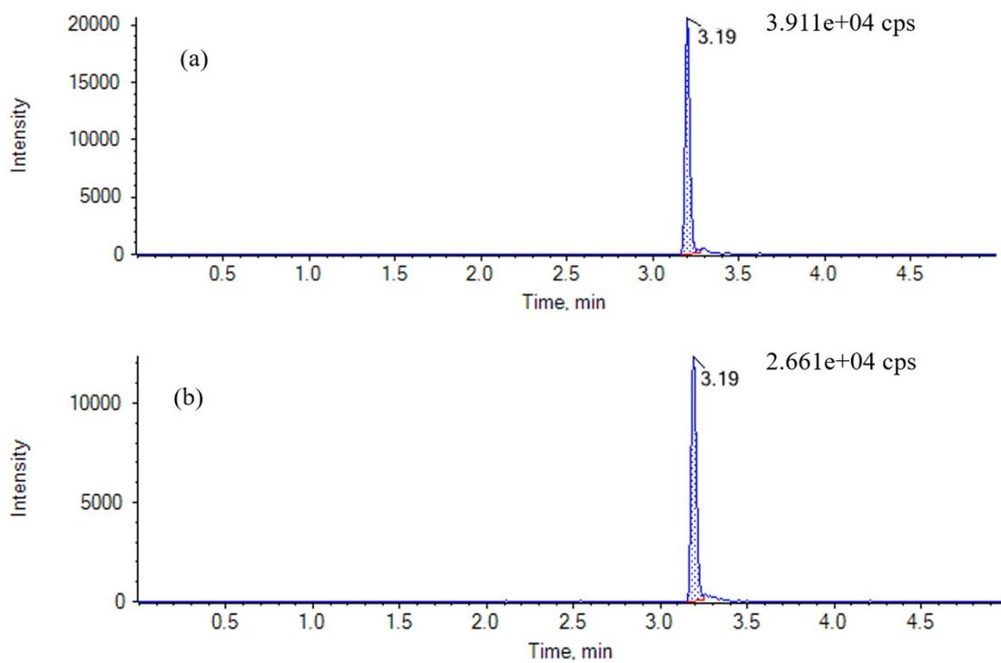
Fig. S5. The MRM chromatograms of the milk samples spiked at the  $50 \text{ ng g}^{-1}$  level of CAP and measured by LC-MS/MS-IAC and LC-MS/MS-SPE (The peak area signals are shown on the graphs)
