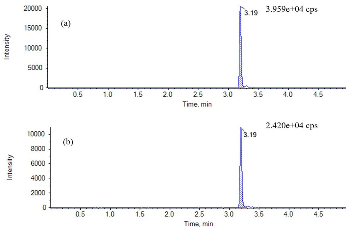
Fig. S4. The MRM chromatograms of the feed samples spiked at the  $50 \text{ ng g}^{-1}$  level of CAP and measured by LC-MS/MS-IAC and LC-MS/MS-SPE (The peak area signals are shown on the graphs)
