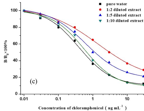
Fig. S2. Matrix effect of shrimp, feed and milk samples on the standard curves of the ELISA for CAP detection. (a) Standard curves of the ELISA for CAP performed in pure water and 1 : 2, 1 : 5, 1 : 10 extracts from shrimp sample, (b) standard curves of the ELISA for CAP performed in pure water and 1 : 2, 1 : 5, 1 : 10 extracts from feed sample, (c) standard curves of the ELISA for CAP performed in pure water and 1 : 2, 1 : 5, 1 : 10 extracts from milk sample
