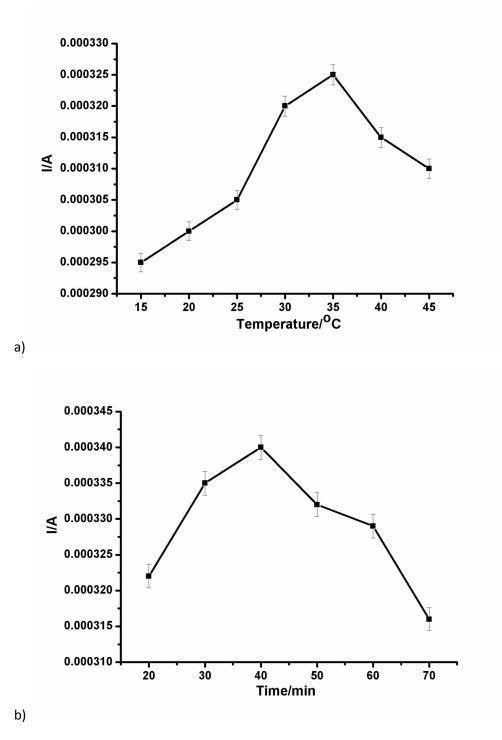
Optimisation parameters of AFP detection Supp. Fig. (1a) Incubation Temperature (1b) Incubation Time.
