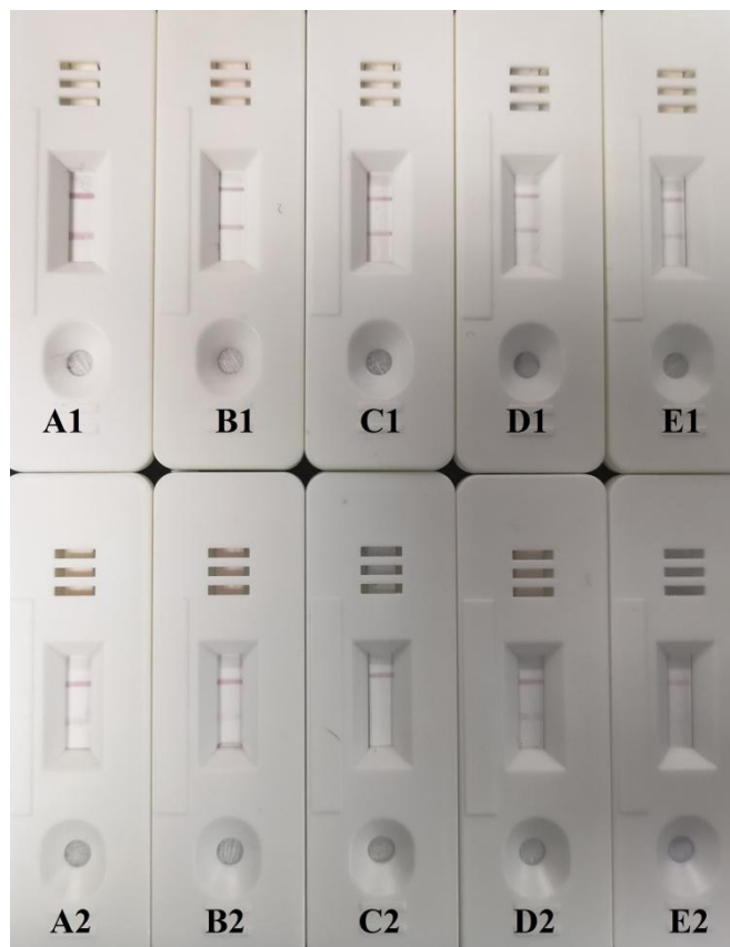
ESM. 2 Results of optimization of diluted times for coating antigen and second antibody (Dilution times T line/C line: A: 10/20; B: 20/40; C: 40/60; D: 40/40; E: 60/60)
