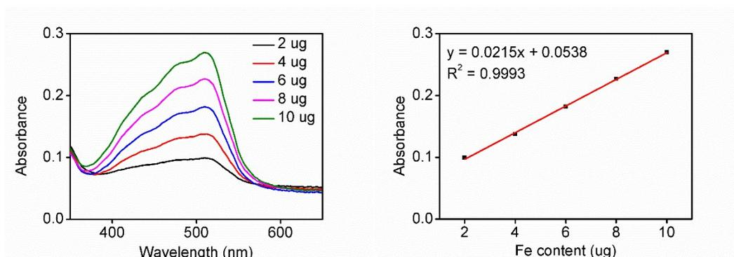
**Figure S18.** Standard absorbance curve of iron content at 510 nm. There were about 0.26 mg eumelanin for per mg Fe.
