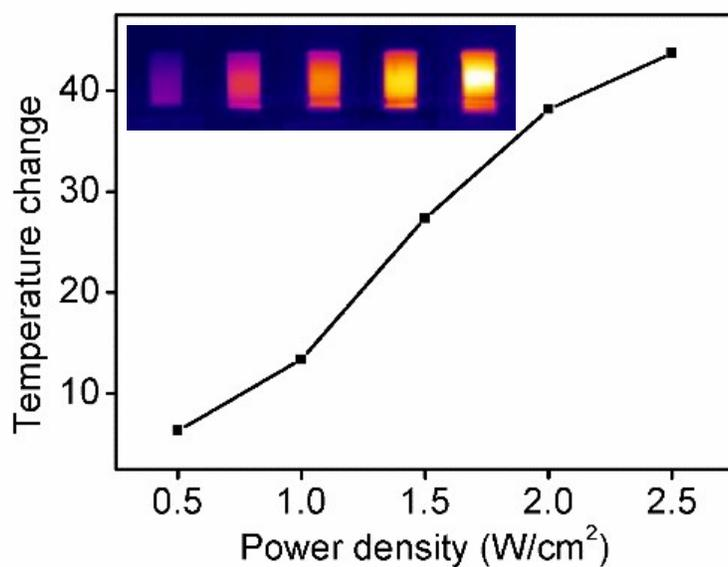
**Figure S10.** Plot of temperature change ( $\Delta T$ ) over a period of 5 min versus power densities.
