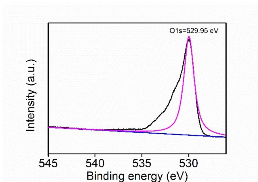
**Figure S7.** O1s spectrum of euMel-Fe<sub>3</sub>O<sub>4</sub> NPs.
