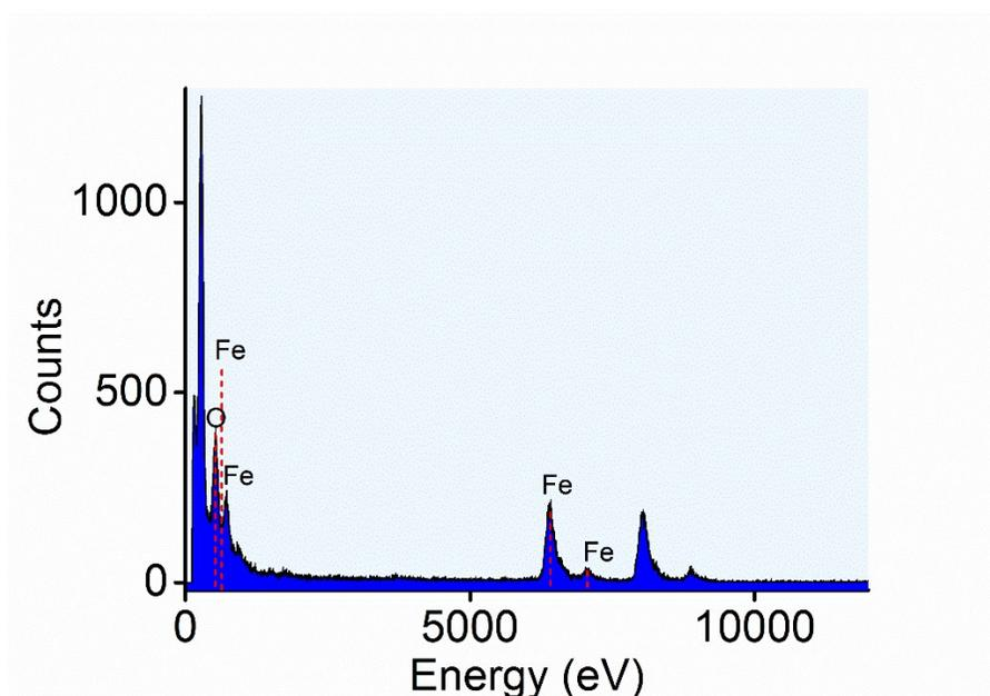
Figure S2. EDX spectrum of euMel-Fe<sub>3</sub>O<sub>4</sub> NPs.
