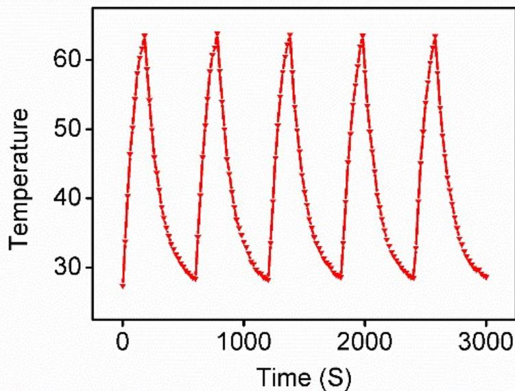
**Figure S15.** Photothermal heating curves of euMel-Fe<sub>3</sub>O<sub>4</sub> NPs (10 mM Fe) irradiated by 808 nm laser at 2 W/cm<sup>2</sup> over five laser on/off cycles (on: 5 min, off: 6 min).
