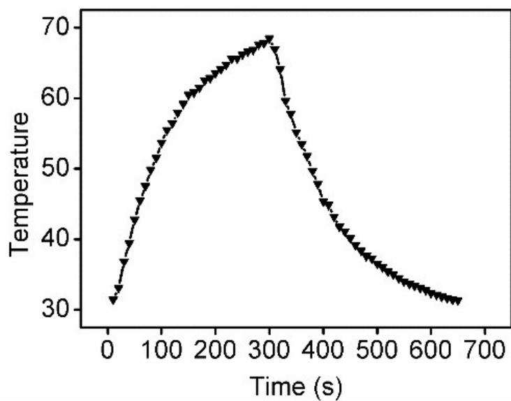
**Figure S14.** Photothermal heating curves of euMel-Fe<sub>3</sub>O<sub>4</sub> NPs (10 mM Fe) irradiated by 808 nm NIR laser at 2 W/cm<sup>2</sup> over one laser on/off cycle.
