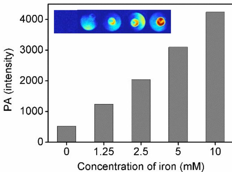
**Figure S11.** The linearity of PA signal intensities under 800 nm laser irradiation as a function of the concentration of euMel-Fe<sub>3</sub>O<sub>4</sub> NPs.
