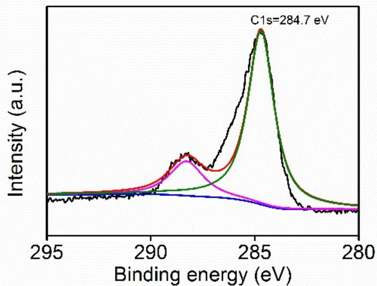
Figure S5. C1s spectrum of euMel-Fe<sub>3</sub>O<sub>4</sub> NPs.
