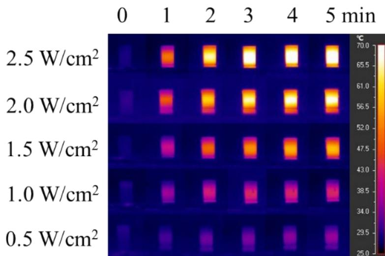
**Figure S8.** Infrared thermal images of euMel- $\text{Fe}_3\text{O}_4$  NP aqueous solution (10 mM Fe) exposed to 808 nm laser with different power densities.
