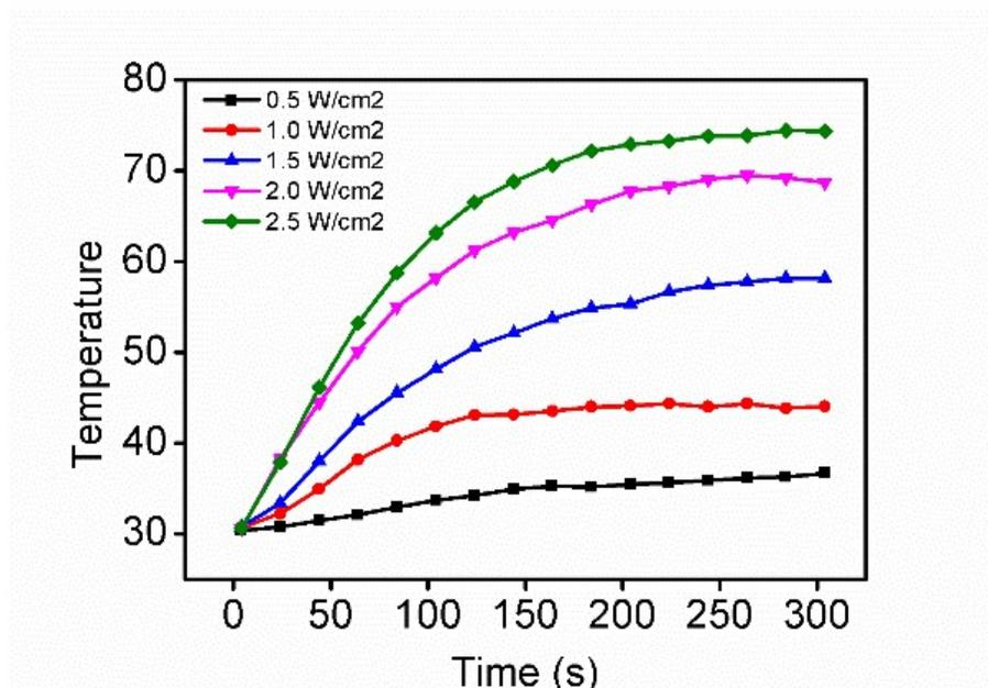
**Figure S9.** Temperature elevation of euMel- $\text{Fe}_3\text{O}_4$  NP aqueous solution (10 mM Fe) exposed to 808 nm laser with different power densities.
