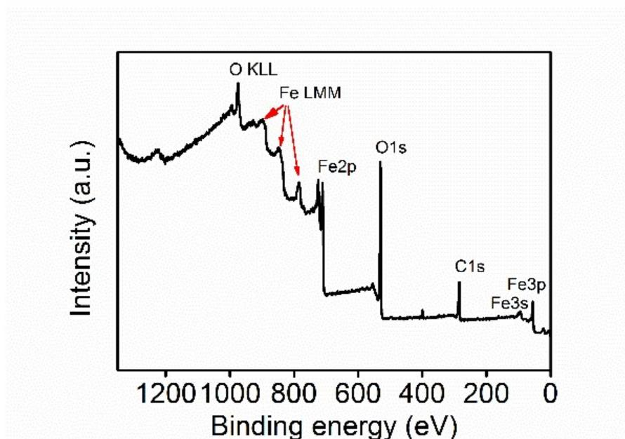
Figure S3. XPS wide scans of euMel-Fe<sub>3</sub>O<sub>4</sub> NPs.
