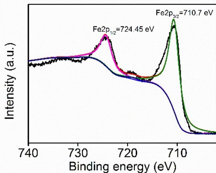
Figure S4. Fe2p<sub>1/2</sub> and Fe2p<sub>3/2</sub> spectra of euMel-Fe<sub>3</sub>O<sub>4</sub> NPs.
