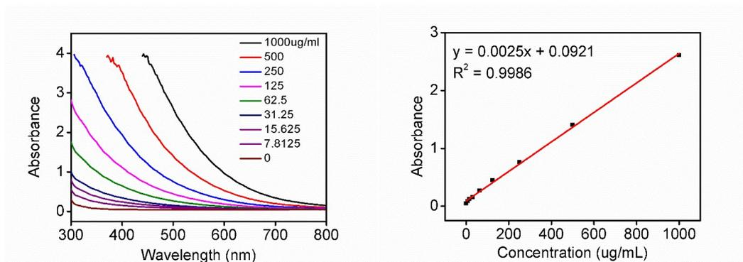
**Figure S17.** Standard absorbance curve of eumelanin solution at 500 nm.
