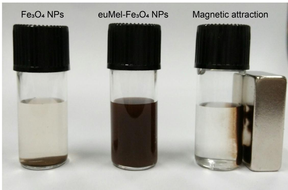
**Figure S1.** Photograph of precipitated pristine Fe<sub>3</sub>O<sub>4</sub> NPs, as-prepared euMel-Fe<sub>3</sub>O<sub>4</sub> NPs in aqueous solution after standing at room temperature for 24 h, and magnetic attraction for euMel-Fe<sub>3</sub>O<sub>4</sub> NPs collection.
