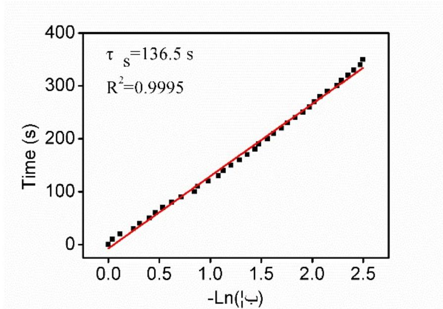
**Figure S16.** Linear time data versus  $-\ln\theta$  obtained from the cooling period. Time constant ( $\tau_s$ ) for heat transfer was determined to be 136.5 s.
