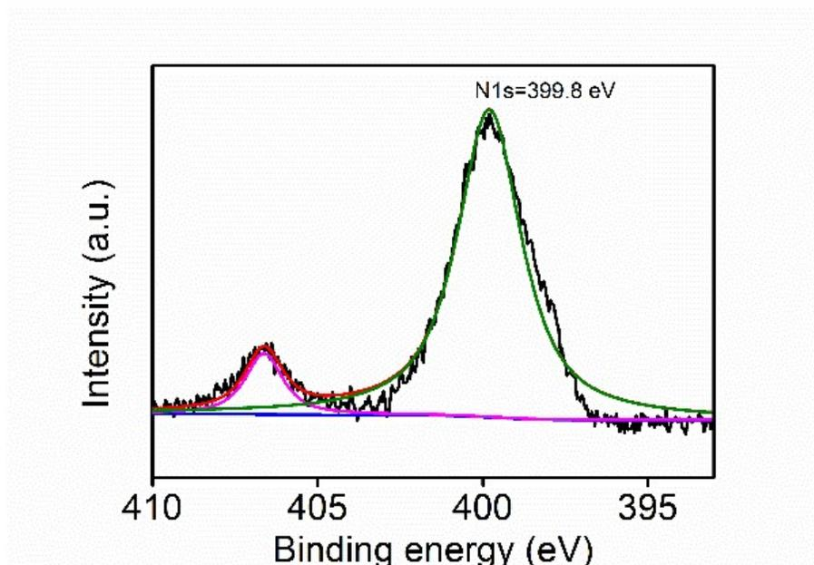
**Figure S6.** N1s spectrum of euMel-Fe<sub>3</sub>O<sub>4</sub> NPs.
