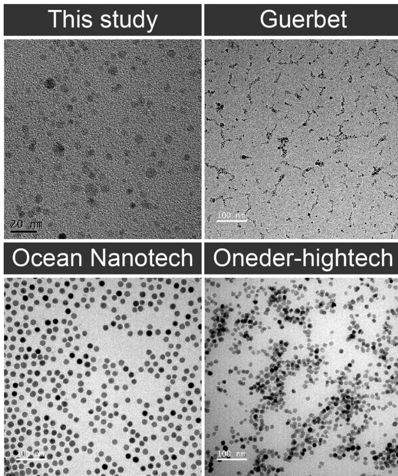
**Figure S12.** TEM image of euMel-Fe<sub>3</sub>O<sub>4</sub> NPs and several commercially available magnetic nanoparticles at equivalent iron molar concentration (10 mM).
