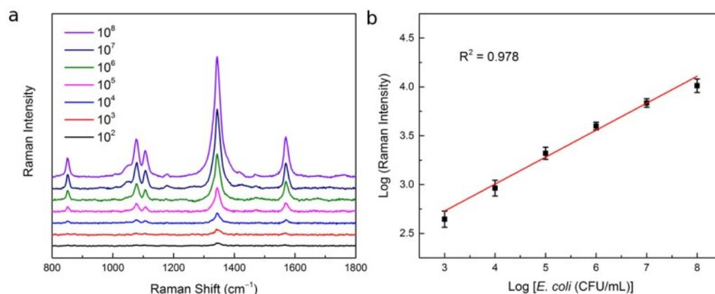
**Fig. S10:** (a) Raman spectra of Man<sub>3</sub>-GNR treated FimH ON bacteria with concentrations from 10<sup>2</sup> to 10<sup>8</sup>. (b) Raman intensity vs. bacterium concentration plot.
