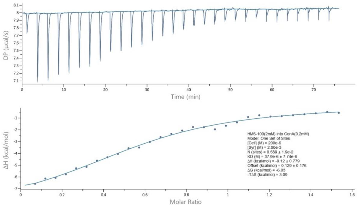
**Fig. S6:** Chromatogram of isothermal calorimetric titration (ITC) of ConA (0.2 mM) with **Man<sub>3</sub>-SH** (2 mM, molar concentration).
