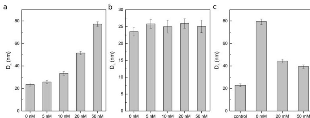
**Fig. S9:** Hydrodynamic diameters of Man<sub>3</sub>-GNR with increasing concentrations of ConA (a), Gal<sub>3</sub>-GNR with increasing concentrations of ConA (b), and Man<sub>3</sub>-GNR with different concentrations of mannose after the addition of 50 nM ConA (c).
