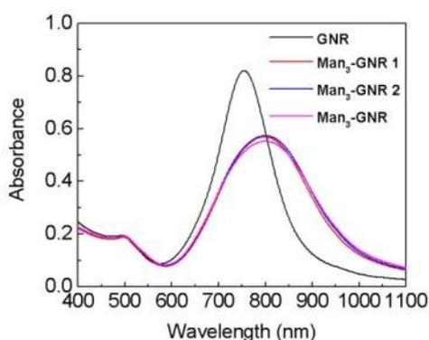
**Fig. S2:** NIR range absorption spectra GNRs and GNRs immobilized with mannose clusters of varied length of thiol terminated linkers and broadening absorption band is due to aggregation of nanorods through ConA recognition with covalently attached tri-thiomannosides.
