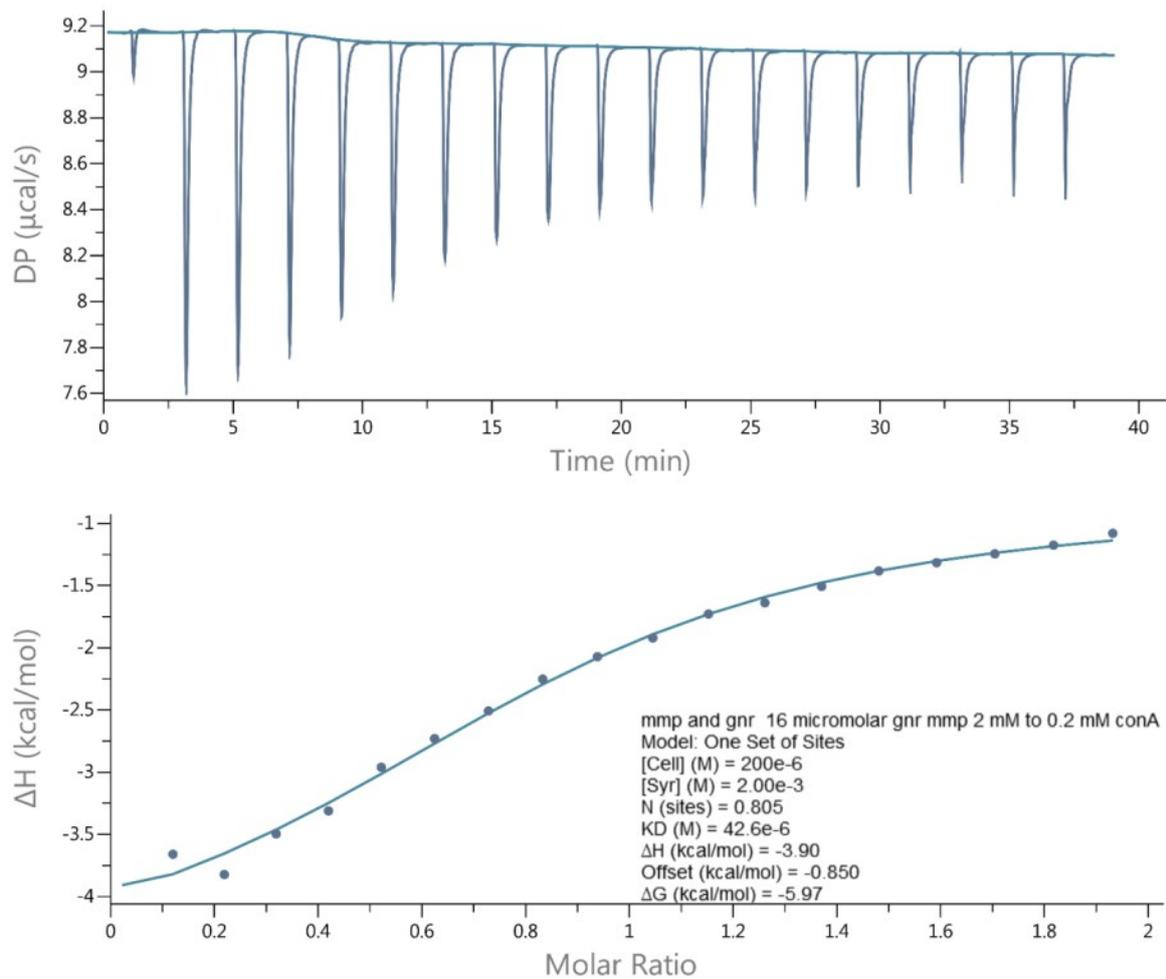
**Fig. S7:** Chromatogram of isothermal calorimetric titration (ITC) of ConA (0.2 mM) with two ligands **Man<sub>3</sub>GNR** (48 μM, mannose basis) and **α-mmp** (2 mM).
