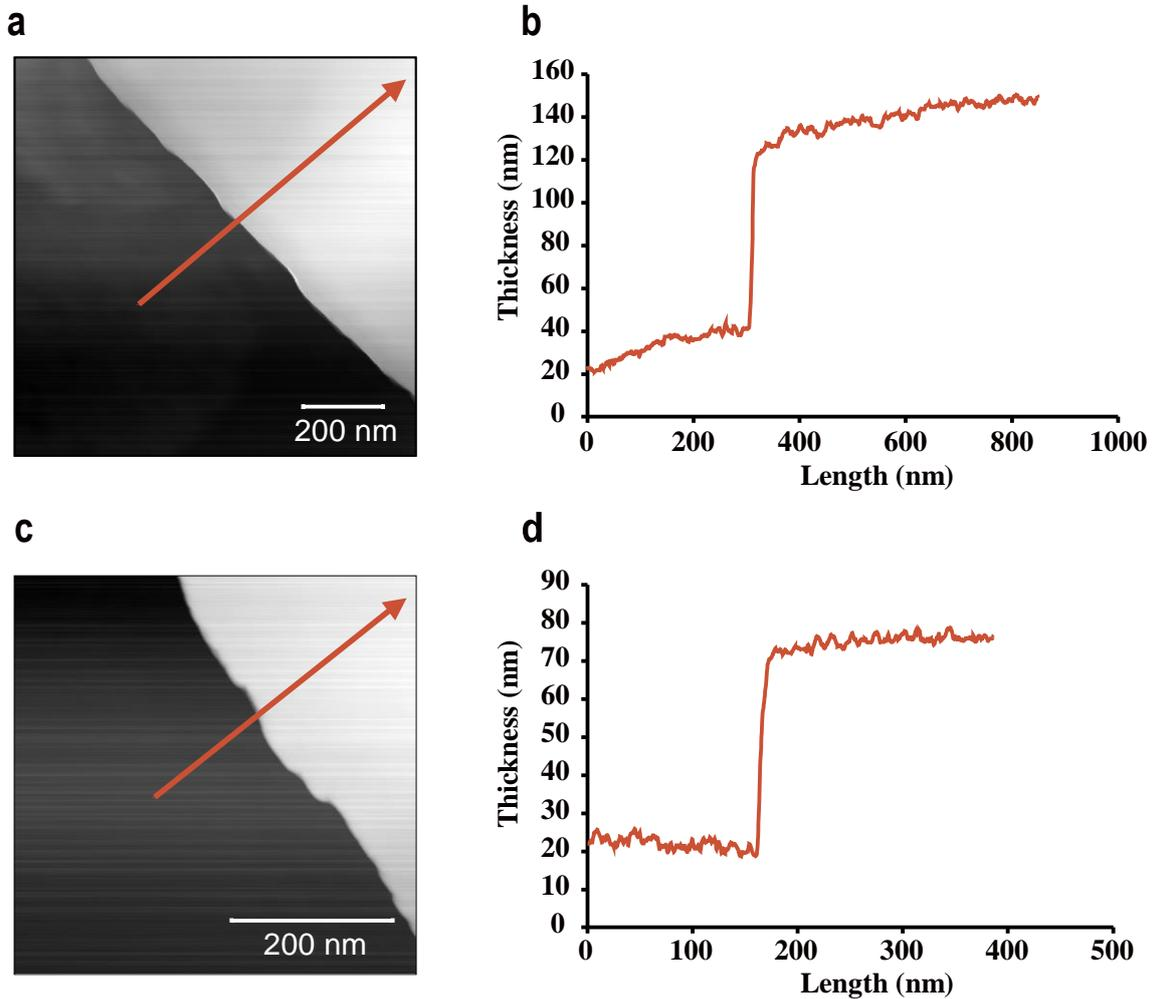
**Supplementary Figure 8. Thickness and surface asperity of the silica film**
