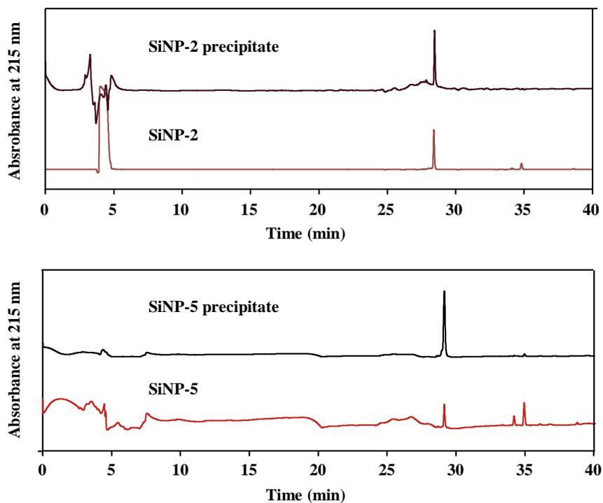
**Supplementary Figure 5. The precipitated silica particles contain SiNP**
