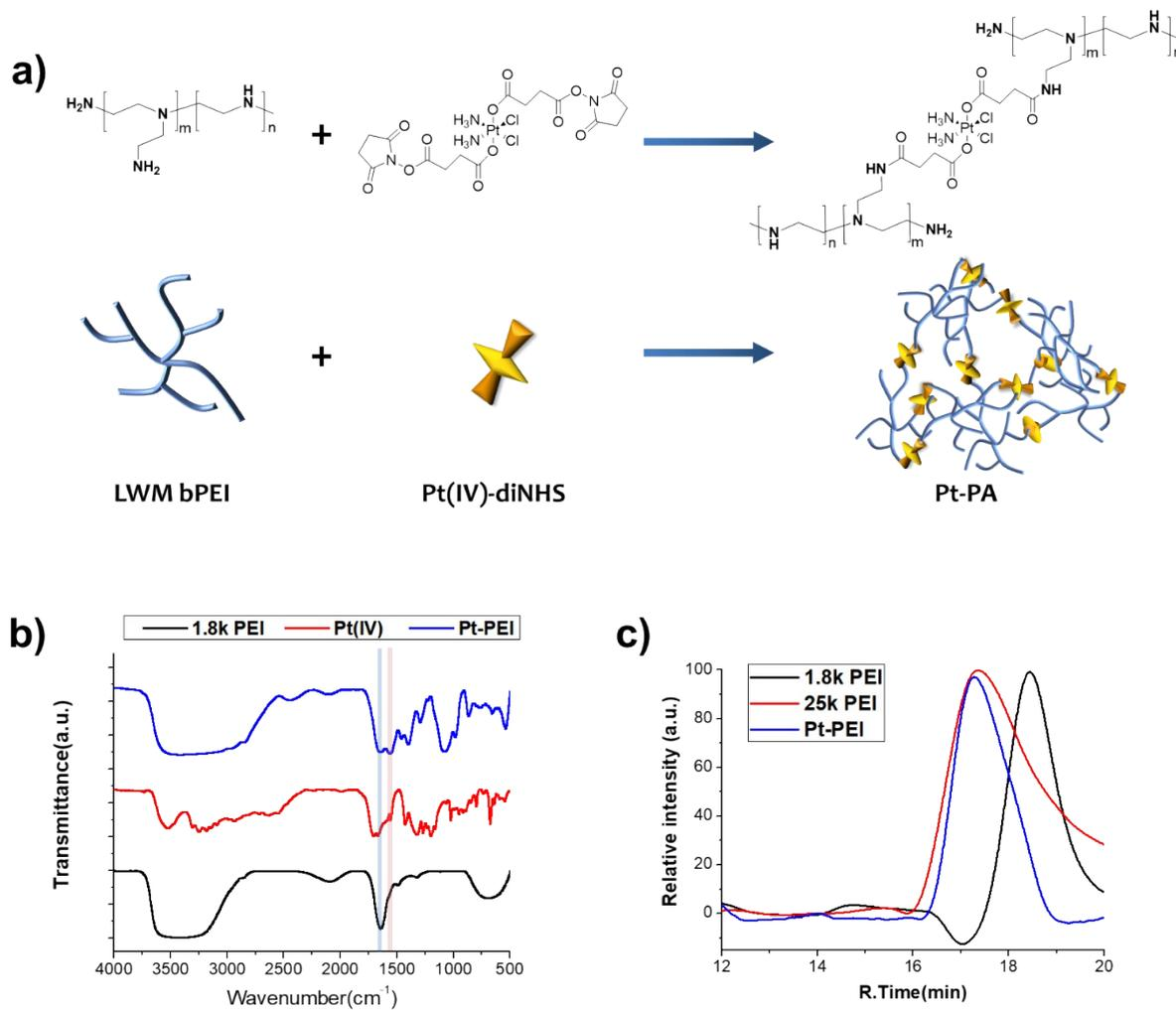
**Figure S4.** (a) Schematic illustration for explanation of polymer crosslinking based on Pt(IV). (b) Formation of amide bond between Pt(IV) and PEI. (c) Normalized intensity of GPC chromatogram depending on the polymer molecular weight.
