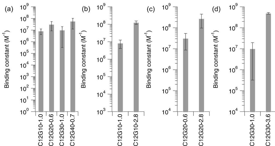
Figure S4 The binding constants ( $K_a$ ) of various amphiphilic glucan dendrimers with TAMRA-BSA (2.5  $\mu$ M). a) The effect of molecular weight of glucan dendrimers on the binding constants, b-d) The effect of the degree of substitution of dodecyl group on the binding constants.
