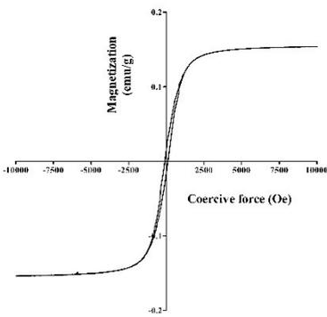
**Figure S3.** The magnetic hysteresis loop of the initial  $\text{Fe}_3\text{O}_4$  nanoparticles.
