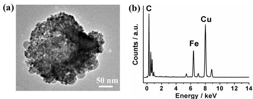
**Figure S6.** (a) TEM image and (b) corresponding EDS result of the adopted MNPs.
