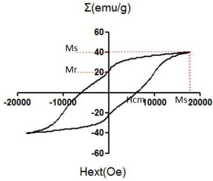
**Figure S2.** The magnetic hysteresis loop of the initial  $\text{Nd}_2\text{Fe}_{14}\text{B}$  particles.
