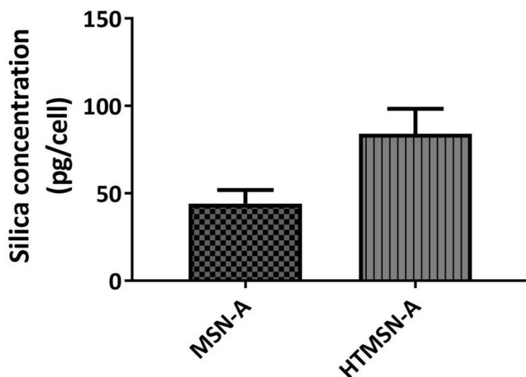
**Figure S7.** Cellular uptake performance of MSN-A and HTMSN-A measured by ICP-OES.
