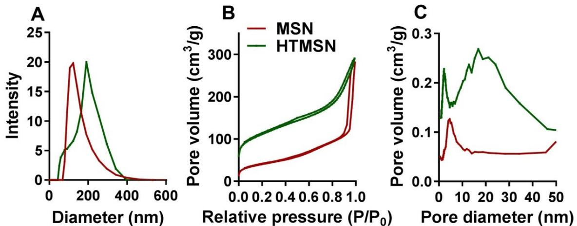
**Figure S1.** A) particle size, B) Nitrogen adsorption-desorption isotherms, and C) pore size distribution of MSN and HTMSN, respectively.
