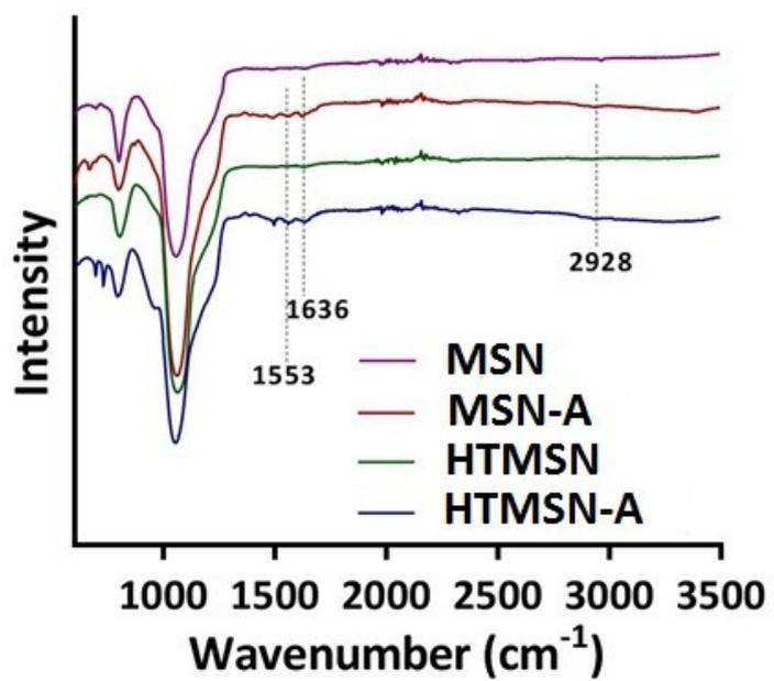
**Figure S3.** FTIR of MSN and HTMSN before and after amino modification.
