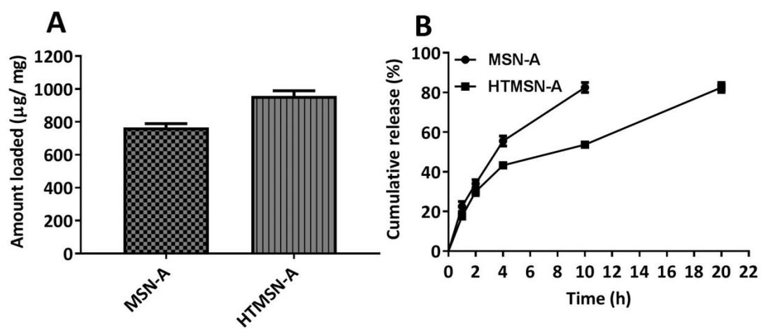
**Figure S5.** A) Loading, B) release of J8 from MSN-A and HTMSN-A.
