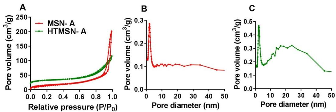
**Figure S2.** A) Nitrogen adsorption-desorption isotherms of MSN-A and HTMSN-A, and pore size distribution of B) MSN-A and C) HTMSN-A, respectively.
