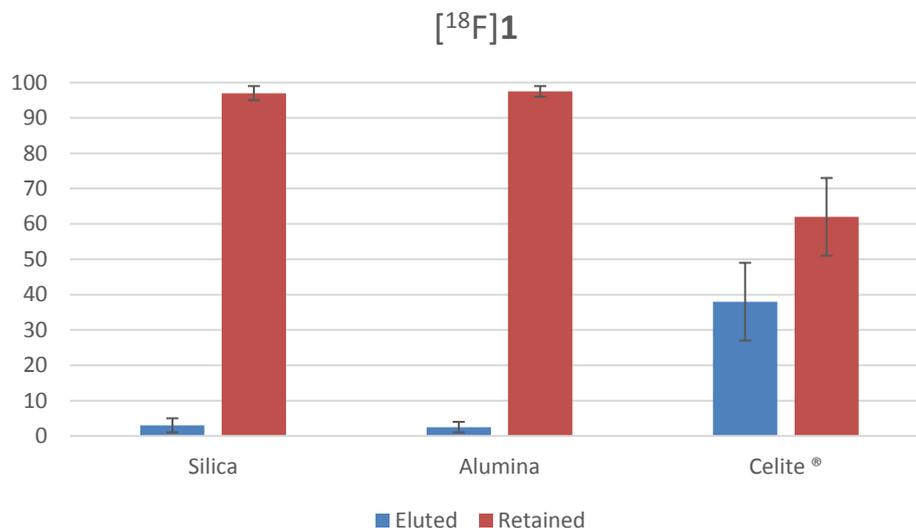
**Figure S6.** Elution of [ $^{18}\text{F}$ ]**1** using diverse adsorbents.
