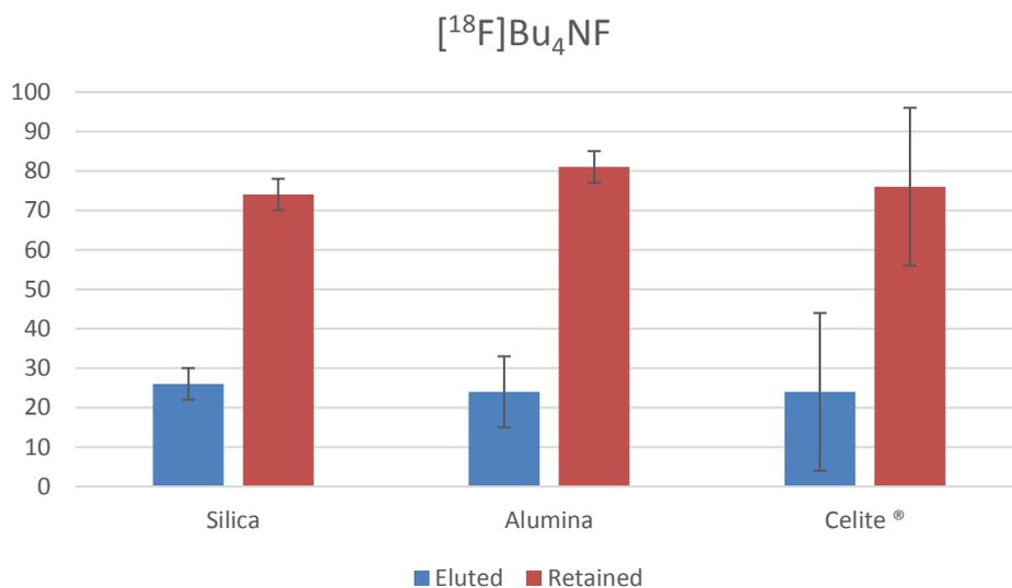
**Figure S7.** Elution of  $[^{18}\text{F}]\text{Bu}_4\text{NF}$  using diverse adsorbents.
