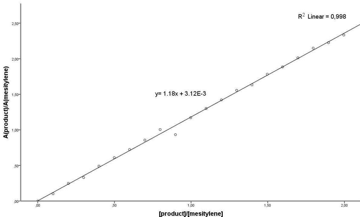
**Figure S1.** GC-calibration curve for oxazolidinone/mesitylene standard ratio.
