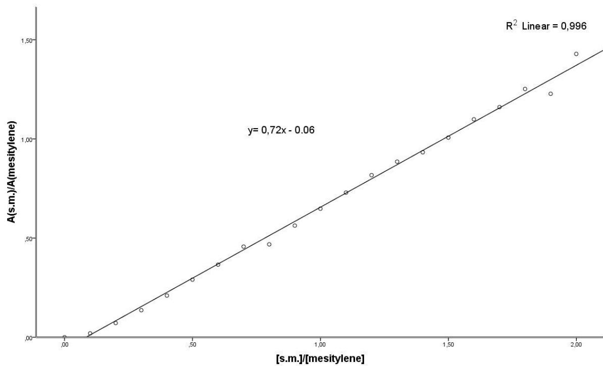
**Figure S2.** GC-calibration curve for aminoalcohol/mesitylene standard ratio.
