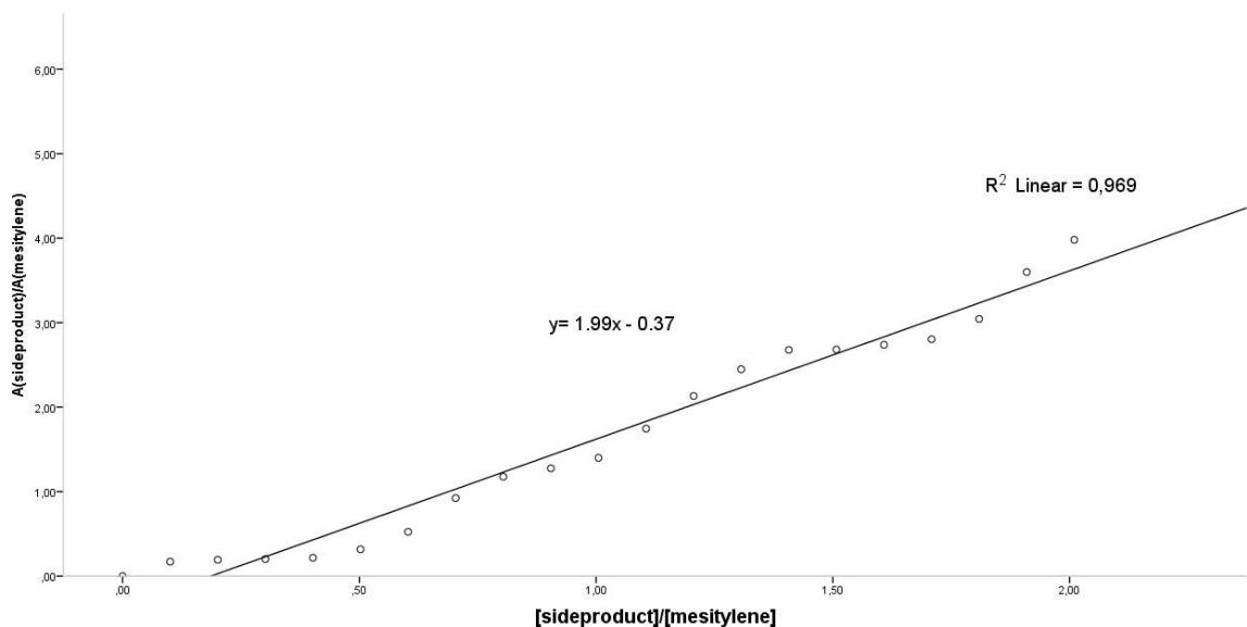
**Figure S3.** GC-calibration curve for the N-tosylated sideproduct/mesitylene standard ratio.
