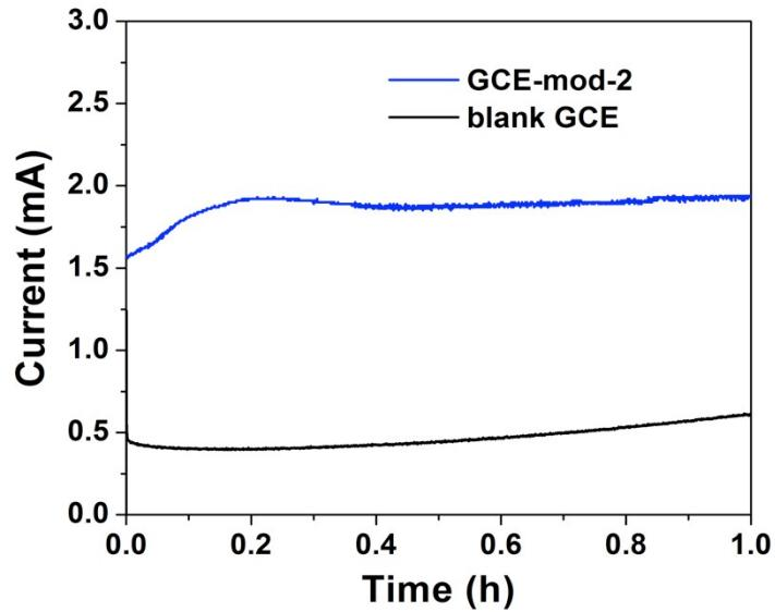
**Figure S13.** Controlled potential electrolysis of mod-GCE-2 (blue) and blank GCE (black) in CO<sub>2</sub> saturated solution of 0.1 M TBAPF<sub>6</sub>/MeCN with 20% water.
