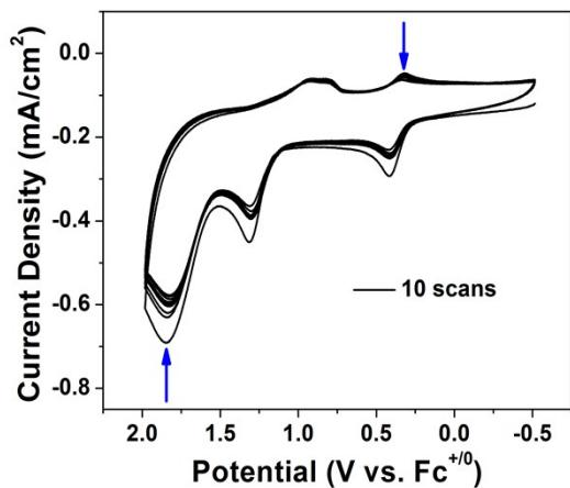
**Fig. S10.** CV of 0.5 mM [Ni(hexynyl-cyclam)]<sub>2</sub>Cl in 0.1 M TBAPF<sub>6</sub> in DCM. 10 scans. Scan rate 200
