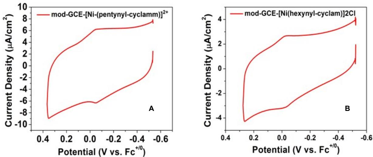
**Fig. S1.** CV of mod-GCE-2 (**A**) and mod-GCE-3 (**B**) in 0.1 M TBAPF<sub>6</sub> in DCM. Scan rate 50 mv/s.
