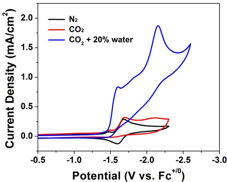
**Fig. S2.** Homogeneous electrocatalysis with 1 mM complex **3** under 0.1 M TBAPF/MeCN with 20% water
