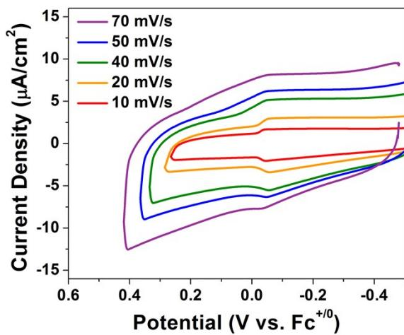
**Fig. S6** Scan rate of mod-GCE-2 in 0.1 M TBAPF<sub>6</sub> in DCM at various scan rates.
