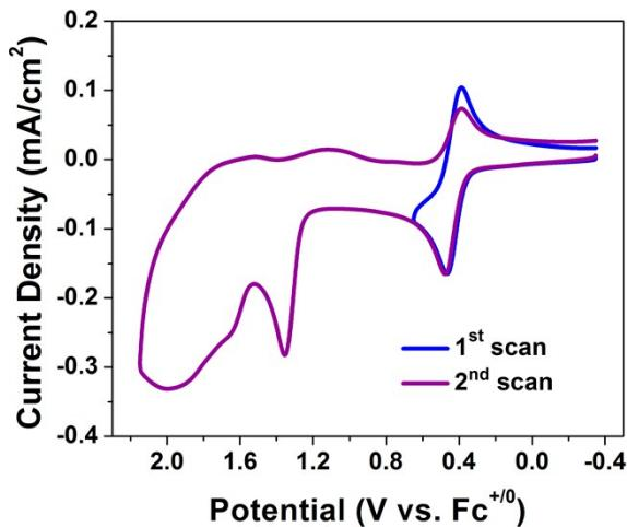
**Fig. S5** CV of 0.5 mM complex **2** in 0.1 M TBAPF<sub>6</sub> in DCM.
