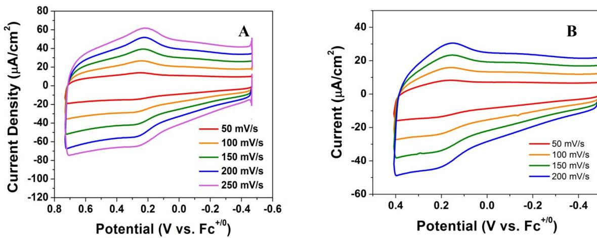
**Figure S11.** Tokai GCE electrodes modified with Ni-alkynyl cyclams. CVs in 0.1 M TBAPF<sub>6</sub> in DCM for the electrode modified with complex **2** mod-GCE-2 (**A**) and with complex **3** GCE-mod-3 (**B**).
