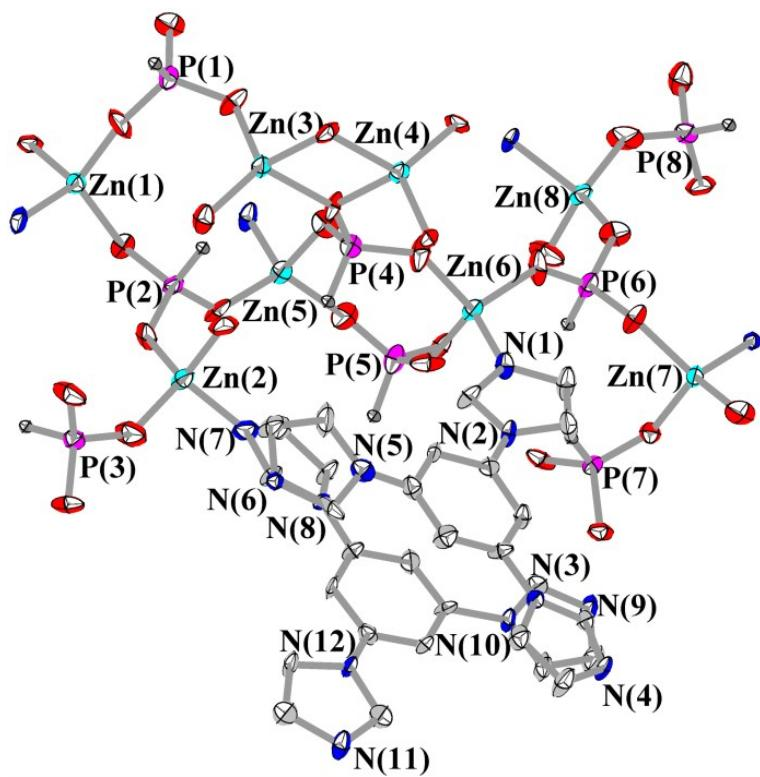
**Fig. S3.** The coordination environment of the Zn atoms in QDU-5.
