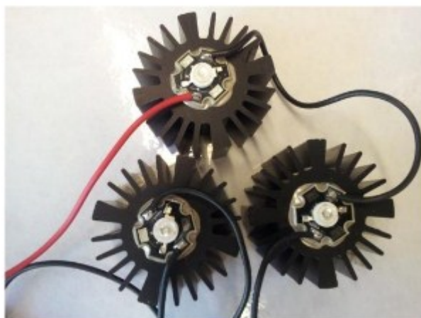
Figure S41: Photograph of the Avonec LED lamps (410-420 nm) (3 x 3 W)
