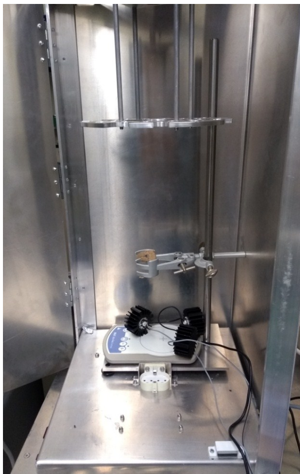
Figure S43: Custom built photoreactor used for the reactions
