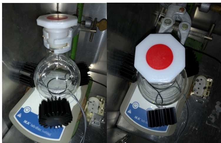
Figure S44: Left: Images of the irradiation setup (frontal and aerial view). Right: Scheme of the geometry of the flask and 3 LED-set-up employed
