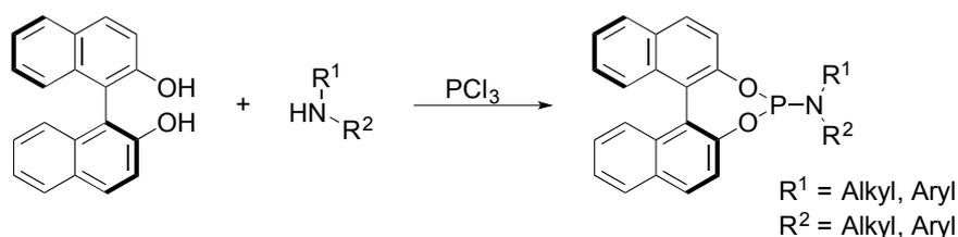
Triethylamine (5.0 eq.) was added dropwise to a stirred, ice-cooled solution of PCl<sub>3</sub> (1.0 eq.) in DCM. The ice bath was removed and the solution left to warm to room temperature
