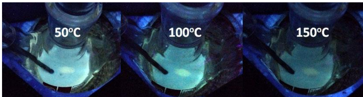
Fig. S5 Digital pictures of Ag: Zn-Ga-S QDs under different heating temperature from 50 to 150 °C under illumination of a UV lamp at 365 nm.
