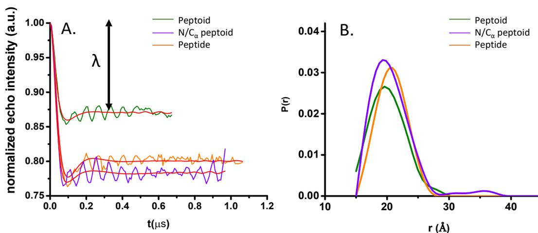
**Figure S5.** Time domain DEER traces after background subtraction with corresponding fits (red) (A) and corresponding distance distributions (B) for pentamer peptoid (green), DS-peptoid (purple) and peptide (orange).
