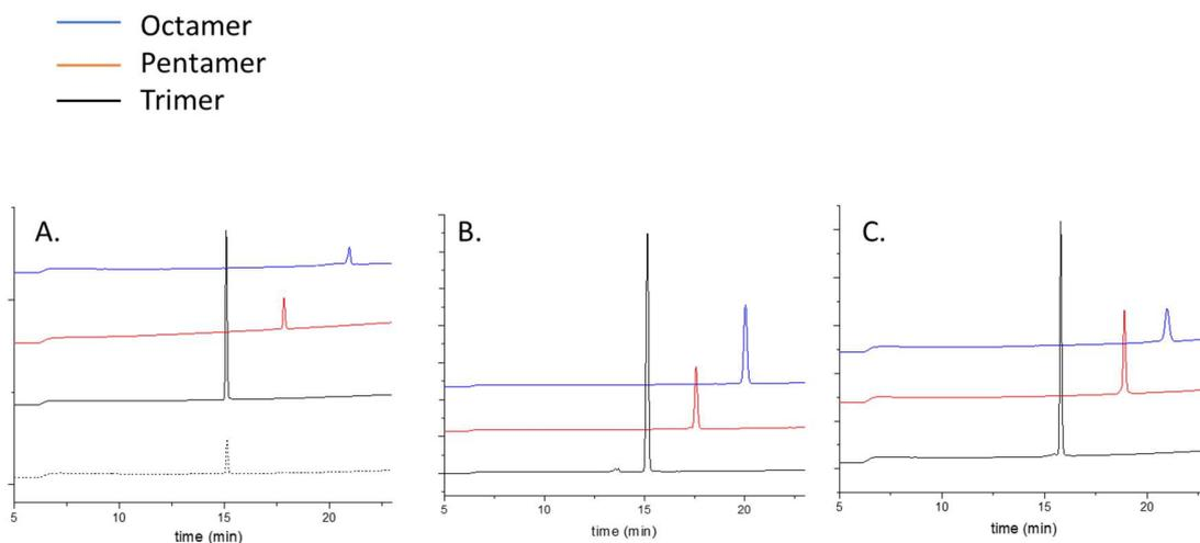
**Figure S2.** HPLC traces at 254nm for the (A) peptide (B) peptoid, and (C) DS peptoid oligomers. Color legend: dashed black; mono-labelled trimer, black; trimers, red; pentamers, and blue; octamers.
