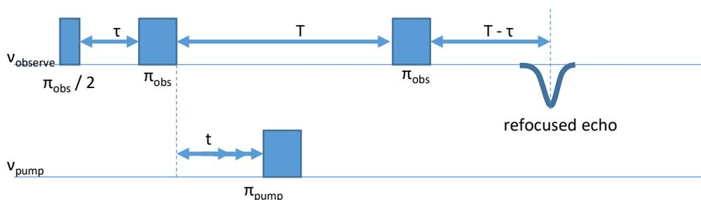
**Figure S3.** Pulse sequence of the 4-pulse DEER experiment.
