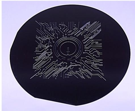
**Figure S10. Precisely designed fine circuit patterns on 4-in. silicon molds by photolithography.**
