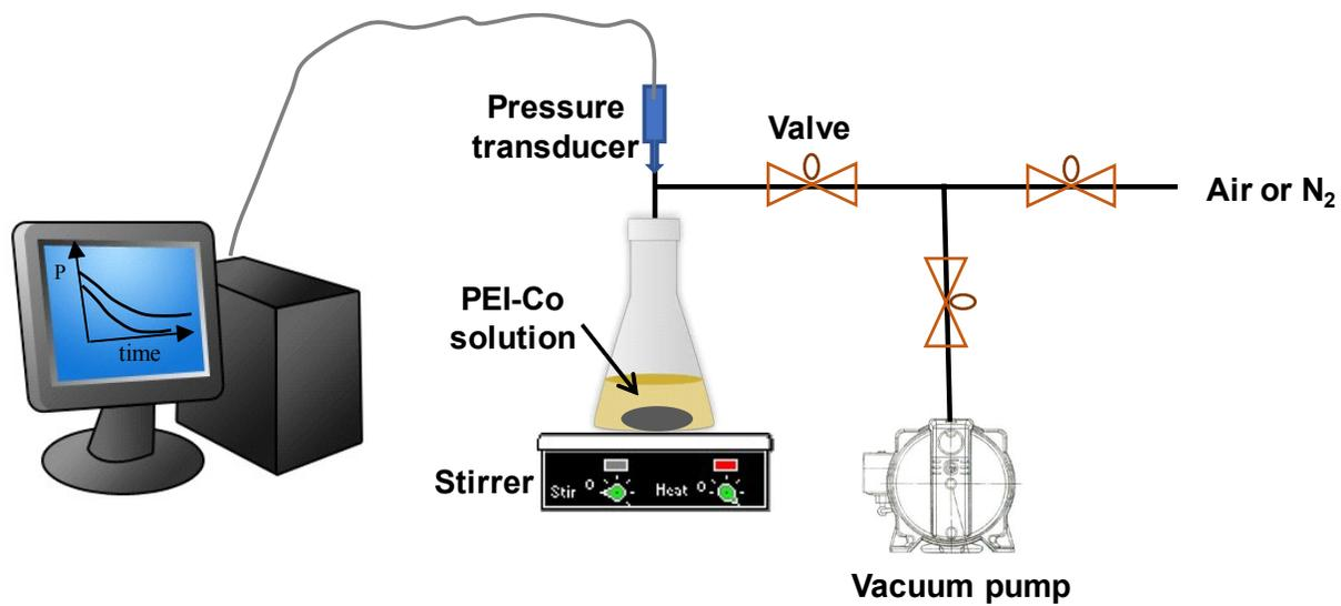
**Figure S1.** Schematic of the system for O<sub>2</sub> absorption capacity and kinetics measurements at room temperature.
