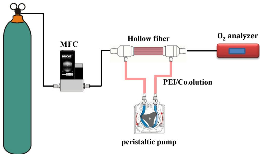
**Figure S2.** Schematic of a flow system for O<sub>2</sub> absorption from air in a membrane contactor.
