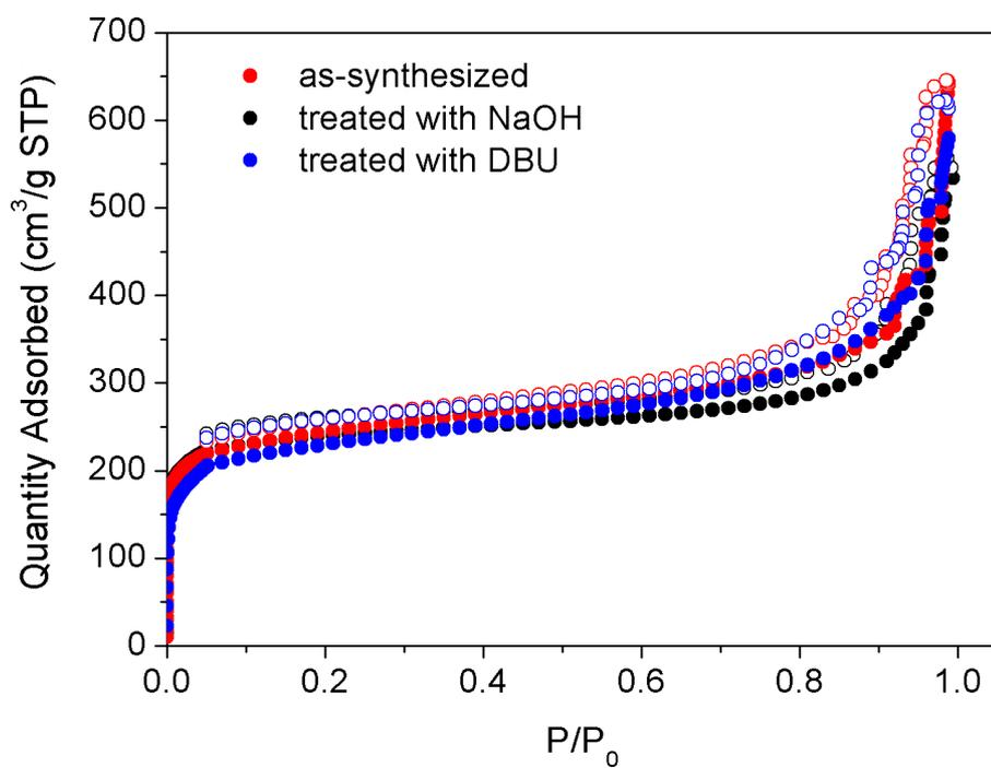
Figure S4. N<sub>2</sub> sorption isotherm of as-synthesized NiBDP-AgS (red), and NiBDP-AgS after treating with pH=13 NaOH aqueous solution (black) and 1M DBU solution (blue).
