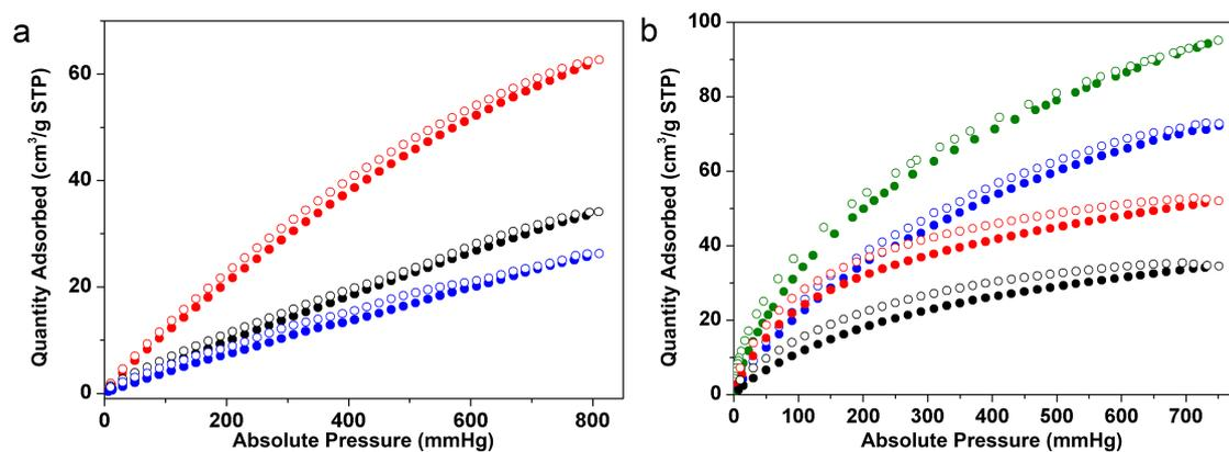
Figure S8. (a) CO<sub>2</sub> sorption isotherms of NiBDP-AgS at 273K (red), 298K (black) and 308K (blue). (b) C<sub>2</sub>H<sub>2</sub> sorption isotherms of NiBDP-AgS at 273K (blue) and 298K (green) and C<sub>2</sub>H<sub>6</sub> sorption isotherms of NiBDP-AgS at 273 (red) and 298K (black).
