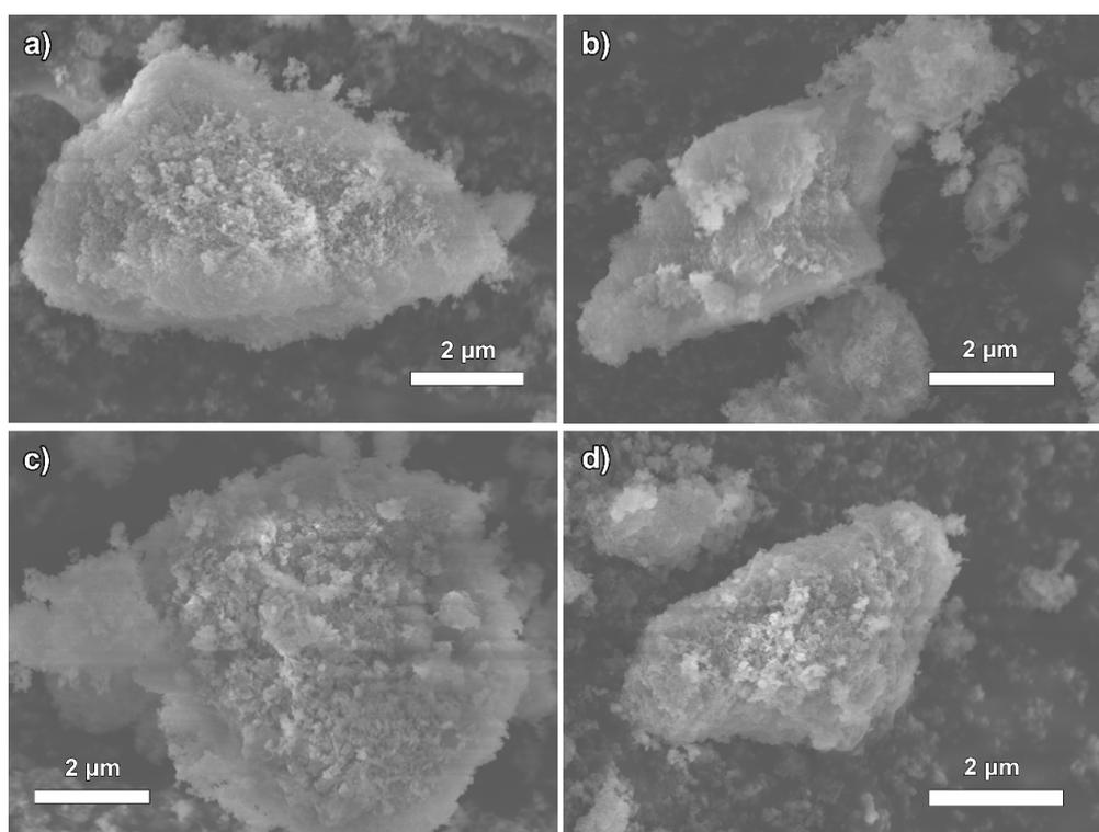
Figure S13. SEM pattern of NiBDP-NH<sub>2</sub> (a), NiBDP-SH (b), NiBDP-AgS (c), and NiBDP-AgS after catalysis (d).
