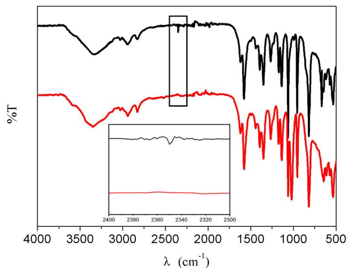
Figure S7. FTIR spectrum of NiBDP-AgS before and after CO<sub>2</sub> adsorption under room temperature and 1 atm.
