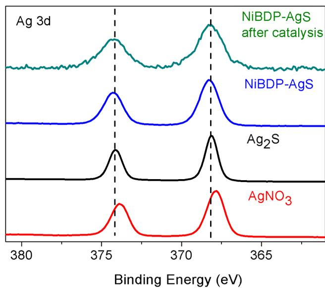
Figure S2. Ag(3d) XPS spectra of AgNO<sub>3</sub>, Ag<sub>2</sub>S, NiBDP-AgS before and after catalysis.
