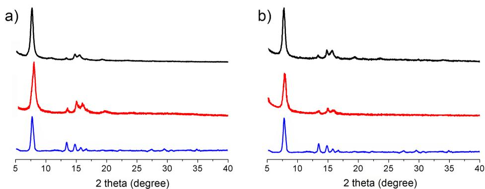
Figure S10. PXRD pattern of as-synthesized NiBDP-AgS (blue), after one-cycle catalysis (red) and ten-cycle catalysis (black) for cyclic carboxylation of propargyl amines (a, left) and cyclic carboxylation of *N*-benzyl-propargylamine (b, right).
