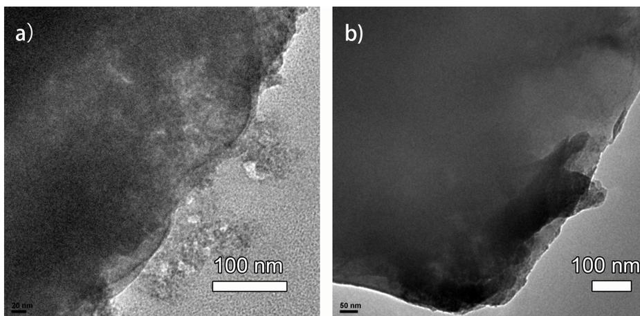
Figure S3. TEM images of NiBDP-AgS before catalysis (a) and after catalysis (b).
