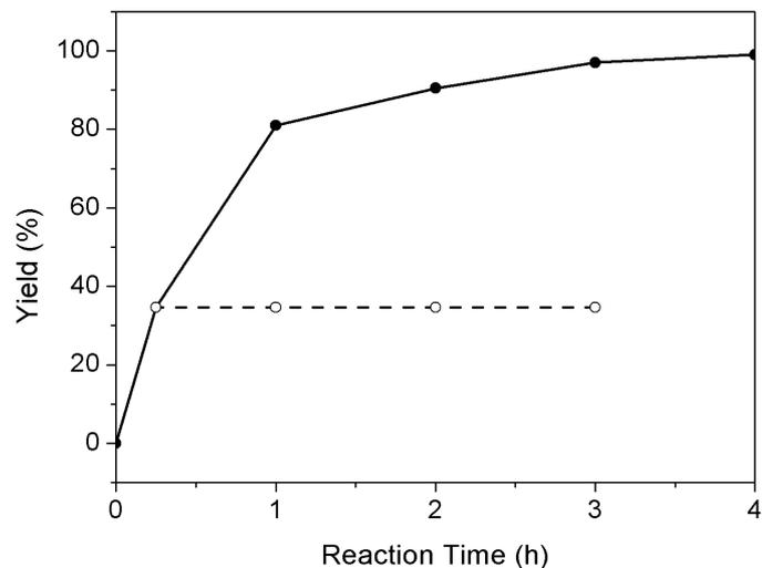
Figure S9. Time-dependent yields of the cyclic carboxylation of *N*-benzyl-propargylamine reaction and the dashed line indicate the reaction yield that the catalyst was removed after the first 15 min of the reaction.
