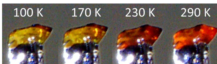
Figure S19. Colour change of a single crystal of (\text{TMA})_2\text{Sn}_3\text{Se}_7 from 100 K to 290 K.
