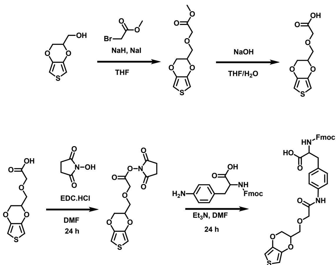
**Fig. S1** Synthesis of the non-natural amino acid Fmoc protected aminophenylalanine coupled to an EDOT molecule (EDOTaa).
