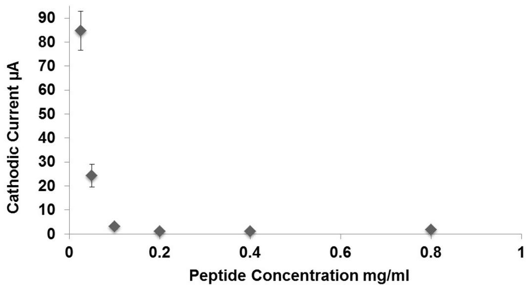
**Fig. S3** Averaged cathodic current after the polymerization of various concentrations of Sequence 2 peptide on a gold electrode. The cathodic current was effectively suppressed above a concentration of  $0.1 \text{ mg mL}^{-1}$  (effective peptide concentration).
