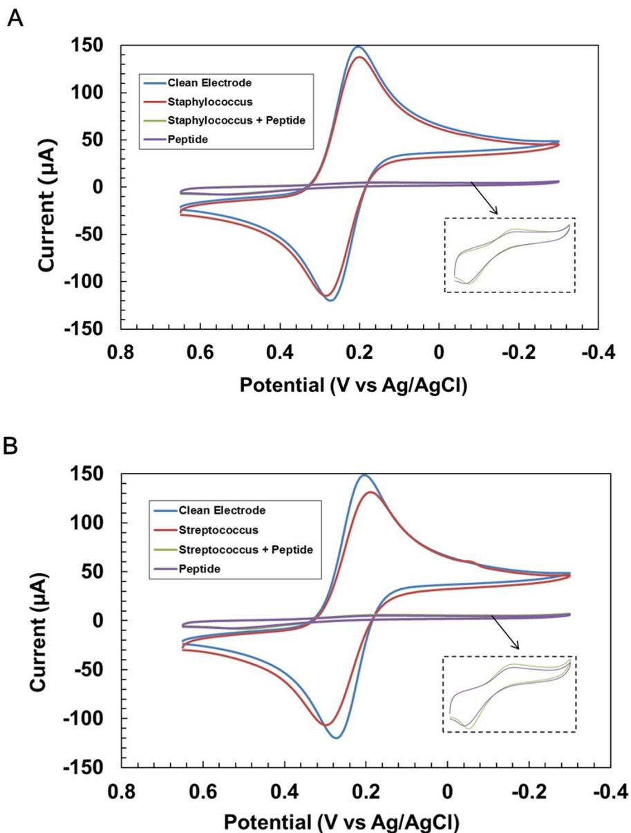
Fig S5. Comparison of cyclic voltammogram (CV) current on a working electrode. CV current on a clean electrode (blue), after polymerization of Sequence 2 peptide in the presence of microorganism (green), only microorganism (red), and only Sequence 2 peptide (purple). (A) *Staphylococcus aureus* and (B) *Streptococcus pneumoniae*.
