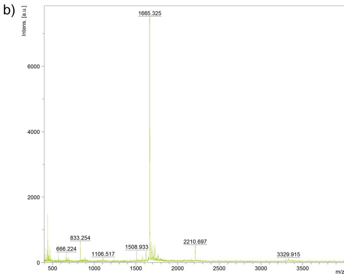
**Fig. S2 Characterization of Sequence 2 peptide** a) HPLC analysis showing the absorbance at 220 nm. b) MALDI MS analysis (Calculated M+H = 1663.99, experimental monoisotopic mass M+H = 1664.32)
