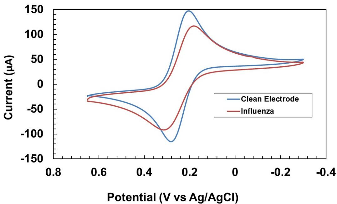
Fig S4. Cyclic voltammogram changes caused by the influenza virus protein. Cyclic voltammograms were measured on a clean electrode, after running the polymerization cycle with  $0.15 \mu\text{g mL}^{-1}$  of influenza virus.
