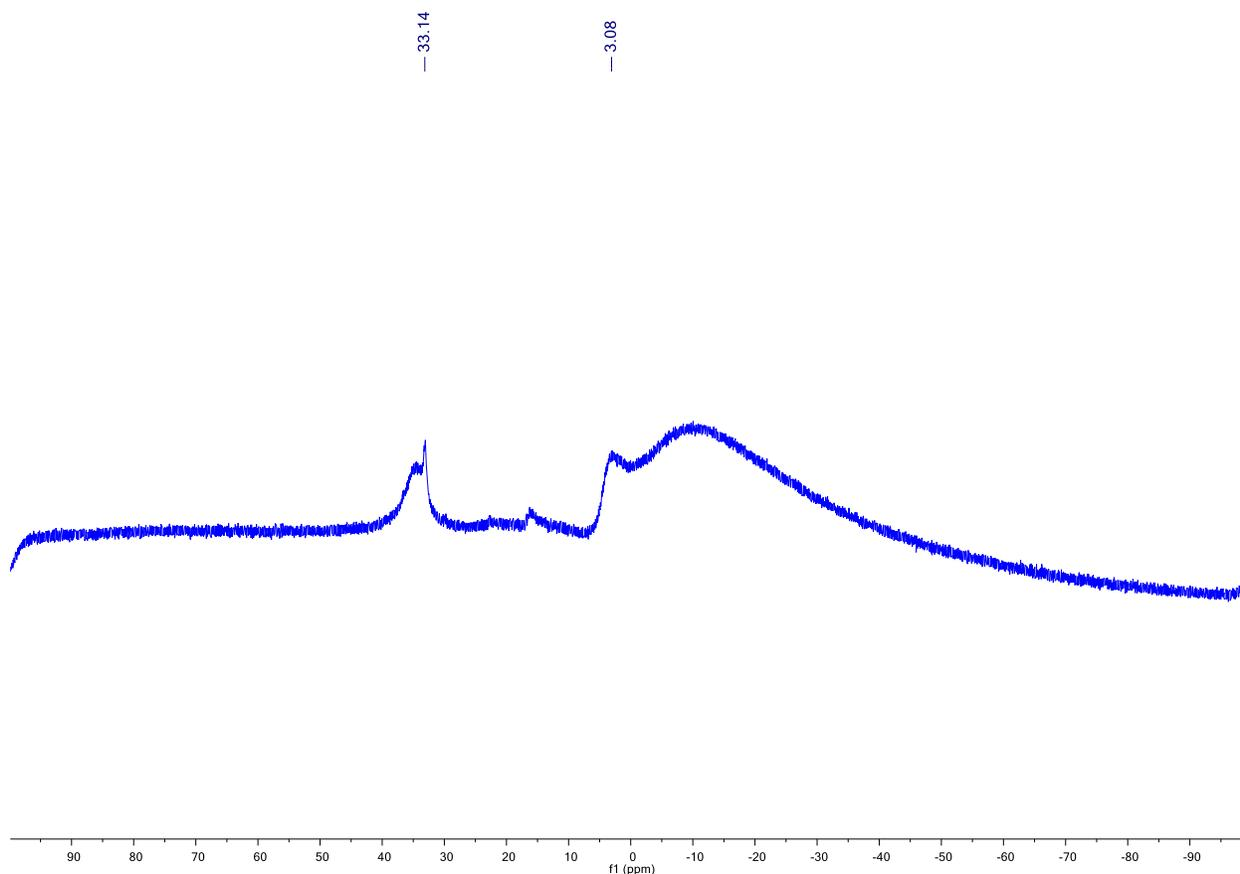
**Figure S3:** In-situ  $^{11}\text{B}$ -NMR for the reduction of **3** by catalyst **7**. The spectrum was acquired at approximately ~20% conversion for the reduction of **3** to **4** and indicates that the catalyst exists as a single major species.
