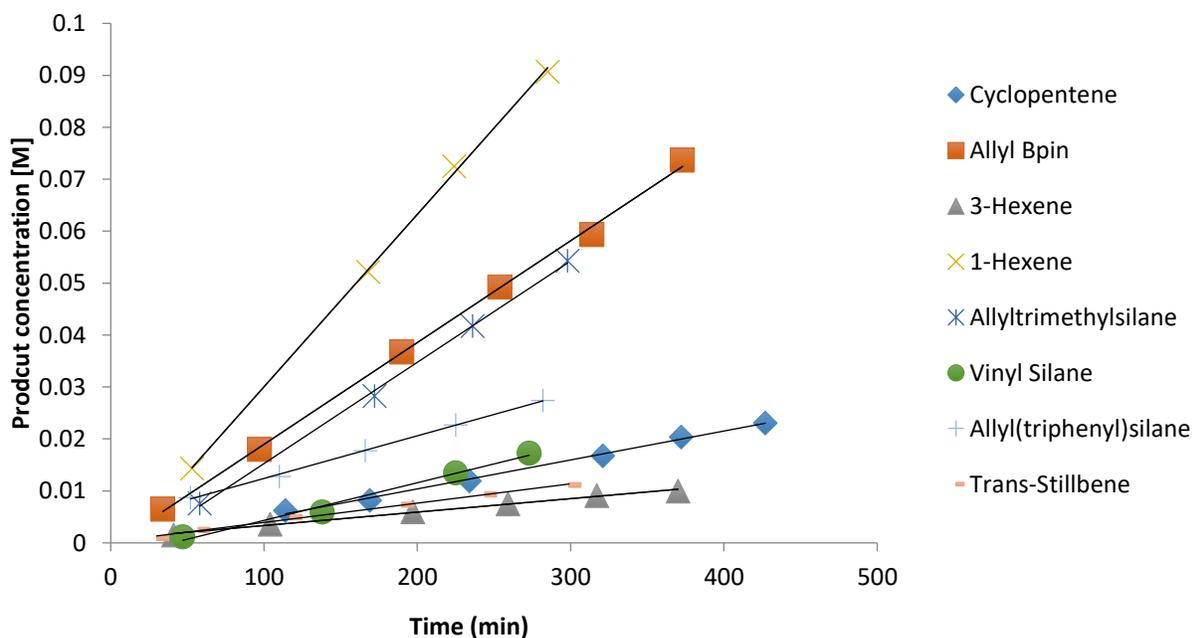
**Figure S1:** Plot for the rate of reduction of **3** to **4** by various *in-situ* derived heteroleptic boron catalysts
