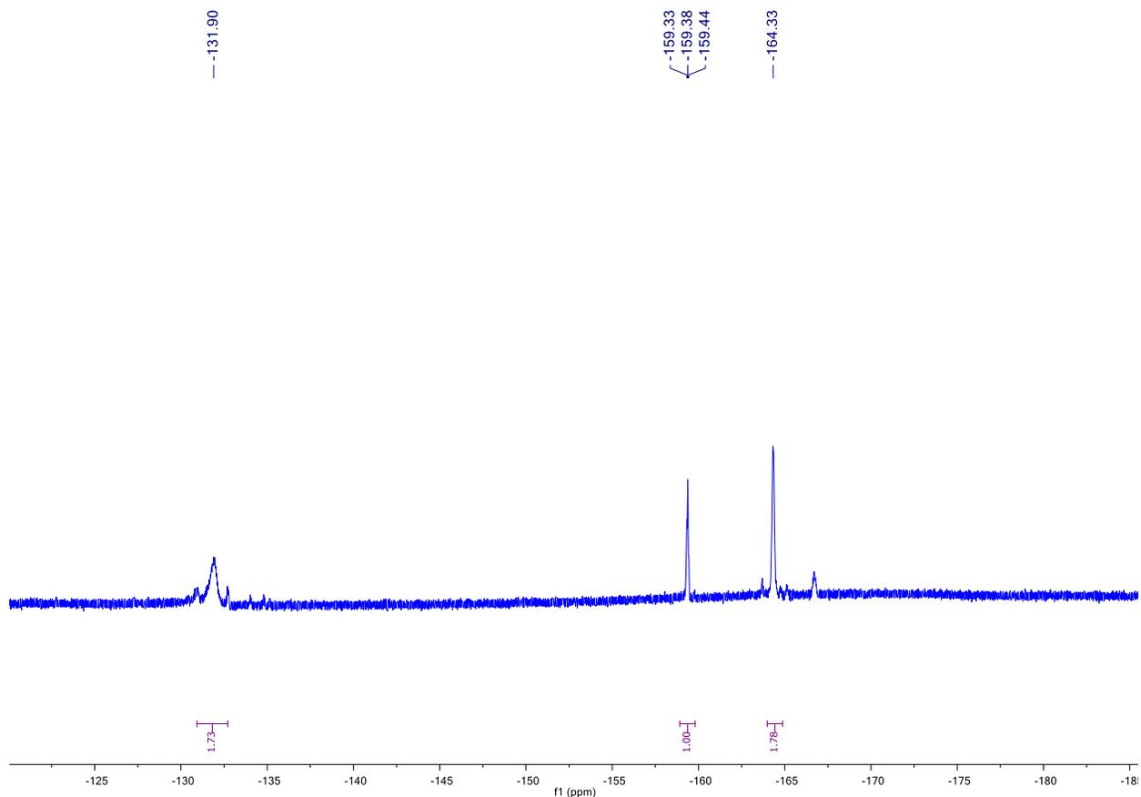
**Figure S2:** In-situ <sup>19</sup>F-NMR for the reduction of **3** by catalyst **7**. The spectrum was acquired at approximately ~20% conversion for the reduction of **3** to **4** and indicates that the catalyst exists as a single major species. The lack of change indicates that under these conditions chain walking of the borane is minimal for catalyst **7**.
