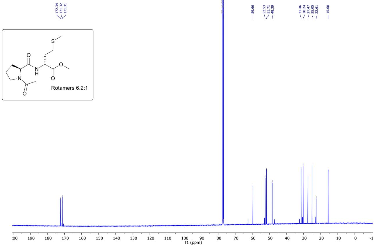
$^1\text{H}$  and  $^{13}\text{C}\{^1\text{H}\}$  NMR of **S20** in  $\text{CDCl}_3$  at  $25^\circ\text{C}$
