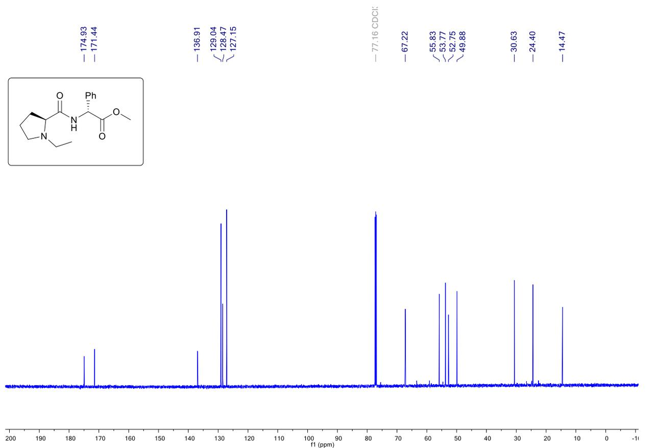
$^1\text{H}$  and  $^{13}\text{C}\{^1\text{H}\}$  NMR of **30** in  $\text{CDCl}_3$  at  $25^\circ\text{C}$ .
