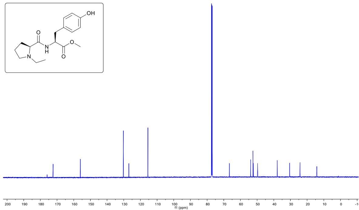
$^1\text{H}$  and  $^{13}\text{C}\{^1\text{H}\}$  NMR of **34** in  $\text{CDCl}_3$  at 25 °C.
