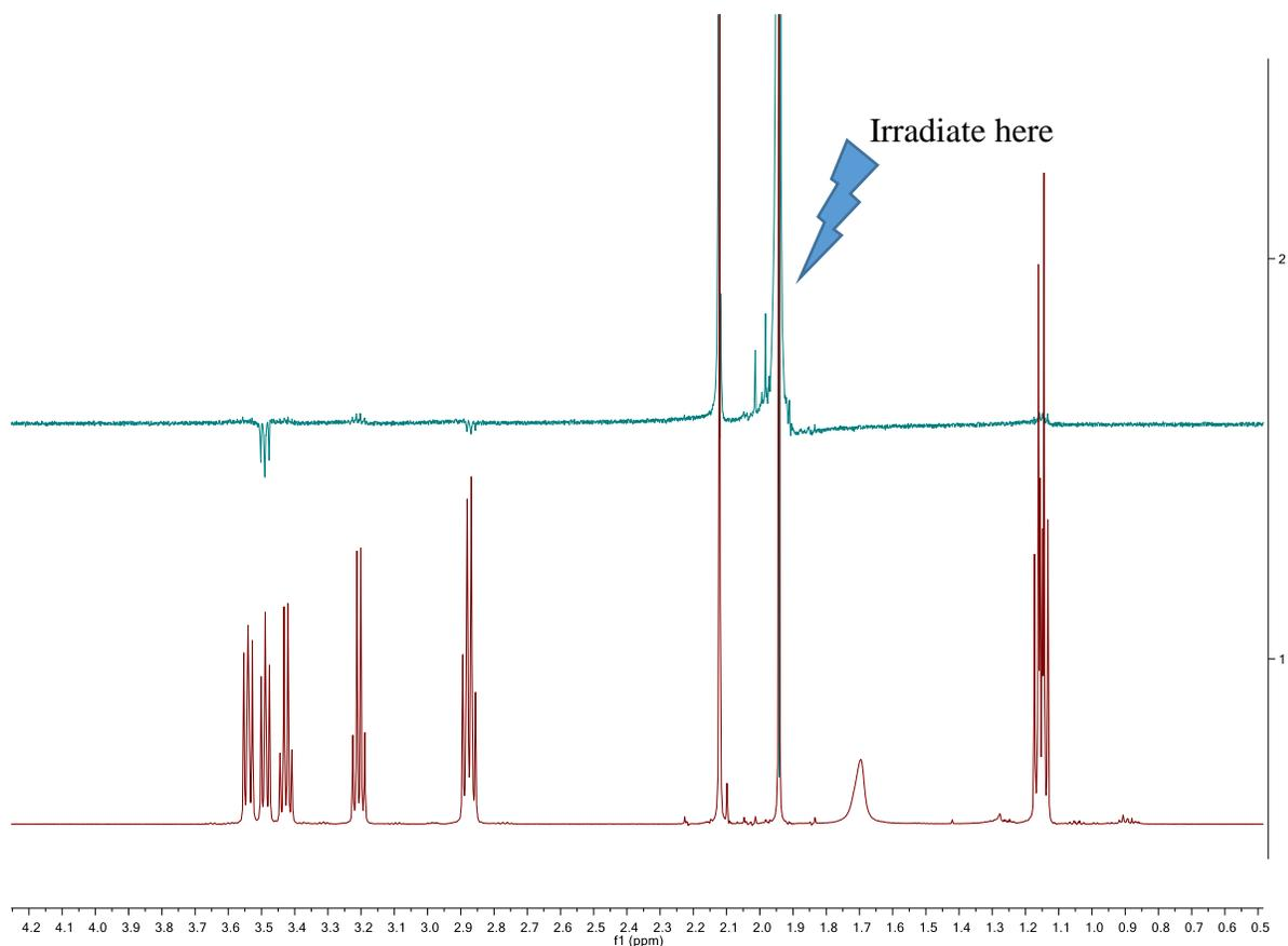
**Figure S3** 1D-NOESY analysis of **S1**. Irradiation of the acetyl group in a 1D-NOE experiment reveals two methyls of the same phase. This suggests the methyl peaks correspond to the two rotamers of **S1**.<sup>3</sup>
