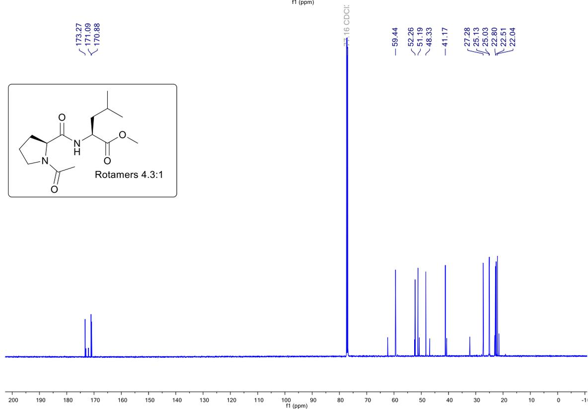
$^1\text{H}$  and  $^{13}\text{C}\{^1\text{H}\}$  NMR of **S22** in  $\text{CDCl}_3$  at 25 °C
