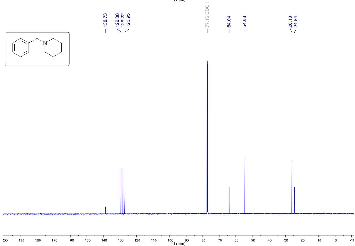
$^1\text{H}$  and  $^{13}\text{C}\{^1\text{H}\}$  NMR of **21** in  $\text{CDCl}_3$  at  $25^\circ\text{C}$ .
