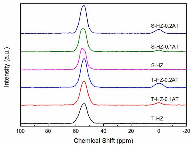
**Fig. S4**  $^{27}\text{Al}$  MAS NMR spectra of HZSM-5 catalysts.
