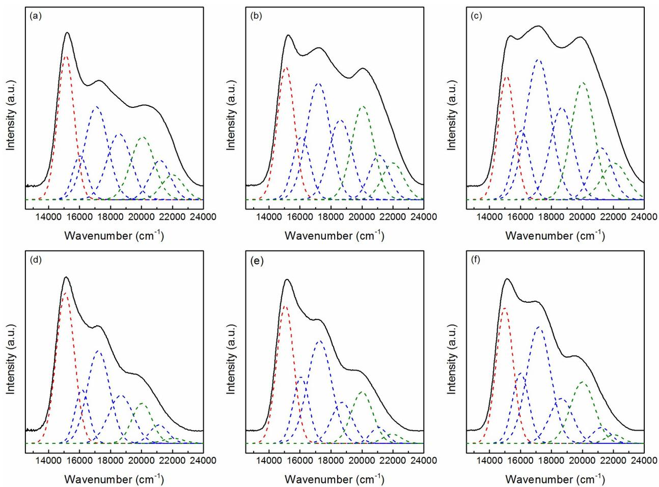
**Fig. S3** Deconvolution of Co(II) UV-vis DRS of Co-ion exchanged (a) T-HZ, (b) T-HZ-0.1AT, (c) T-HZ-0.2AT, (d) S-HZ, (e) S-HZ-0.1AT, and (f) S-HZ-0.2AT.
