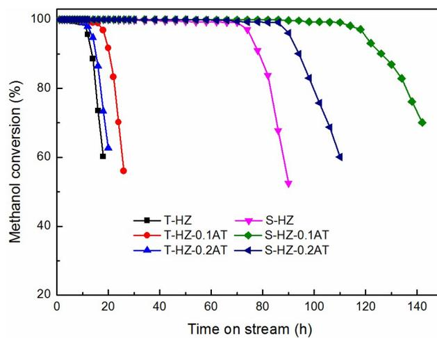
**Fig. S6** Methanol conversion as a function of time on stream for MTP over HZSM-5 catalysts, reaction conditions:  $T = 450\text{ }^{\circ}\text{C}$ ,  $\text{WHSV} = 6\text{ h}^{-1}$ .
